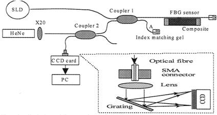
Figure 1 Scnematic illustration of the experimental set-up for the FBG strain measurement experiments.
