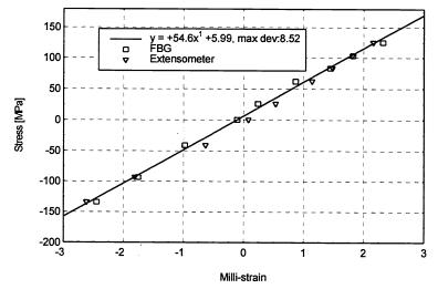
Figure 7 Stress/strain curve after 266,000 cycles obtained with a surface mounted extensioneter and a surface mounted FBG sensor.
