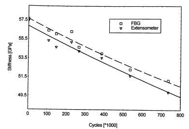
Figure 10 Stiffness-decay data using a surface mounted extensometer and a FBG sensor. The composite was under fatigue testing using a peak stress of 210 MPa, a frequency of 6 Hz and a stress ratio of -0.5.
