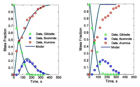
Fig. 3: Comparison of model predictions and experimental data (Wang *et al.*, 2006) at 923K: the multi-stage, multi-reaction model (left), and the reduced, single-reaction version (right).
