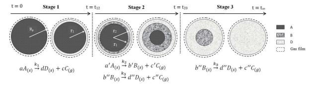
Fig. 1. Schematic of solid particle reaction including intermediate formation.
