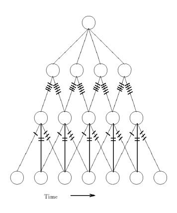
Figure 4: A simplified illustration of the structure of a Time Delay Neural Network (TDNN). Weights with corresponding markings have equal values. Therefore only 9 of the 27 weights shown are independent. The bias weights are not shown. Each node of this diagram would be replaced by a set of nodes in a realistic network.
