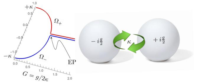
Figure 1. Schematic illustration of a  $\mathcal{PT}$ -symmetric dimer formed by two identical (no frequency detuning) coupled optical resonators, but with opposite values of the gain/loss parameter  $G(=2g/\kappa)$ . In the absence of gain/loss ( $G=0$ ), the two resonators form common hybridized states with splitting by  $2\kappa$ , while for the exceptional point (EP) at  $G=1$ , the system is degenerate, i.e.  $\Omega_+ = \Omega_-$ , with coalescing eigenstates.
