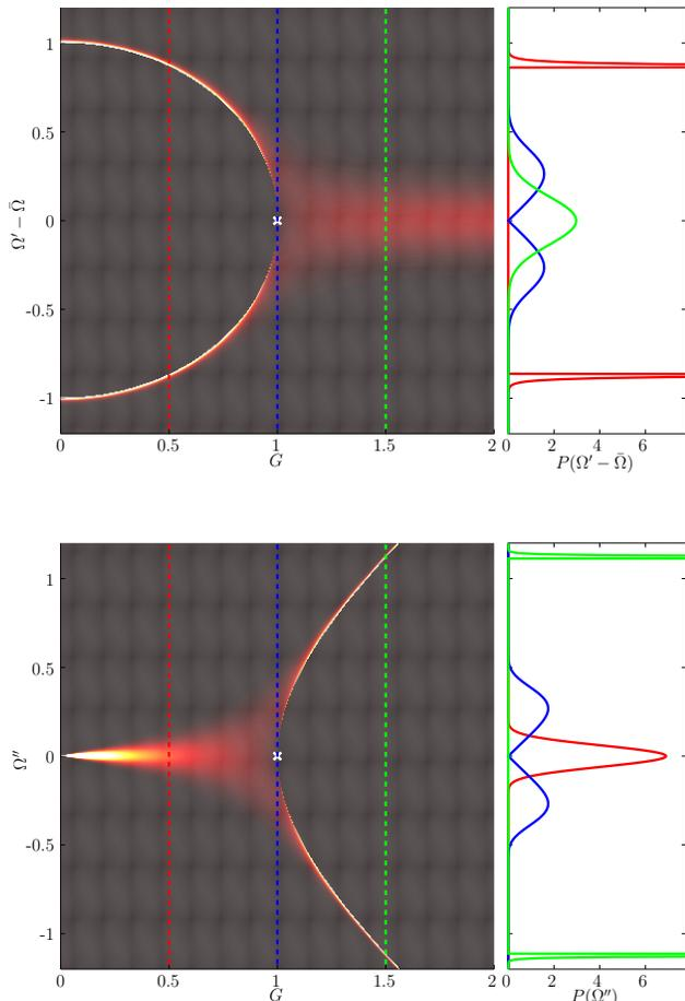
Figure 2. Plots of the distribution of complex eigenfrequencies  $\Omega = \Omega' + i\Omega''$  for varying  $G$ . The upper panel shows  $P(\Omega')$  while  $P(\Omega'')$  is displayed in the lower panel for an ensemble of coupled resonators with  $\sigma = 0.1$ . Clearly, the sample-to-sample fluctuations are pronounced as one approaches the exceptional point.
