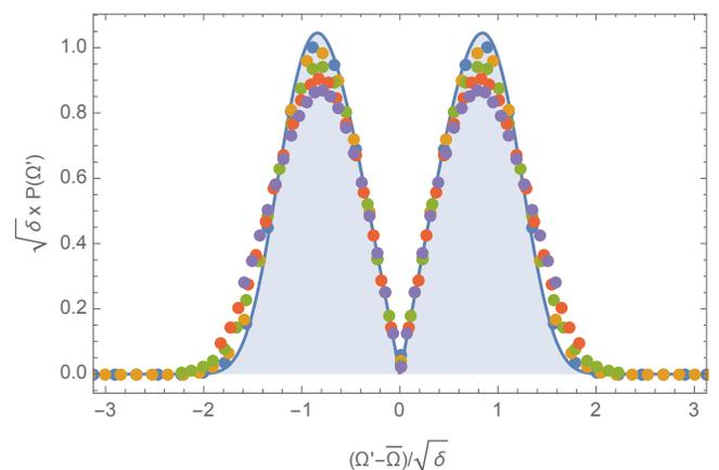
Figure 3. Plot of the distribution of  $P(\Omega')$  versus  $\Omega' - \bar{\Omega}$  at the exceptional point ( $G = 1$ ) for ensembles of coupled resonators with  $\sigma = 0.05, 0.1, 0.2, 0.3$ , and  $0.4$ . Data points are the results of numerical ensemble averaging of the spectra associated with Eq. (2b), while the filled curve shows the approximate universal result from Eq. (8).
