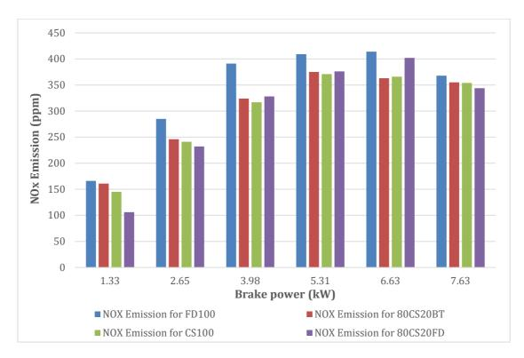
Figure 101: NO<sub>x</sub> emission vs. load of FD100, CS100 and its blends.
