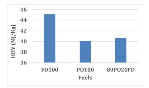
Figure 61: HHV of FD100 with PO100 and its blends.
