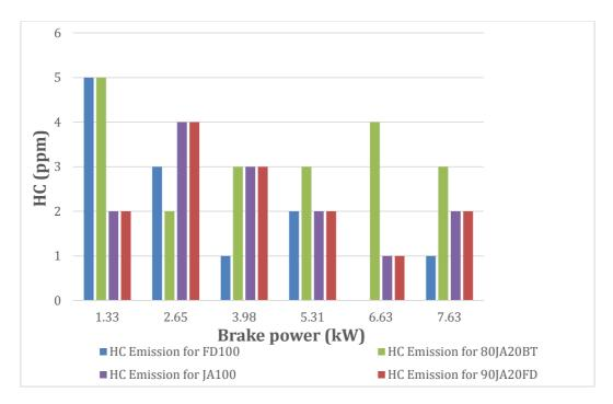
Figure 87: HC emission vs. load of FD100, JA100 and its blends.
