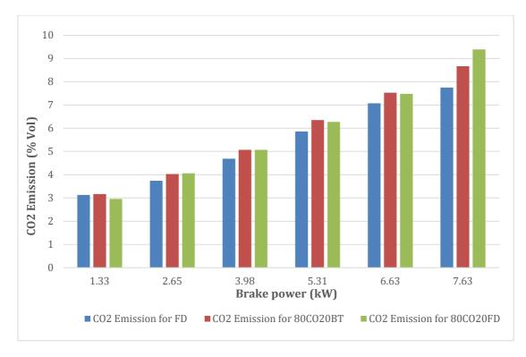
Figure 110: CO2 Emission vs. load of FD100, CO100 and its blends.
