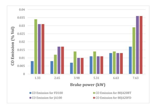
Figure 84: CO emission vs. load of FD100, JA100 and its blends.
