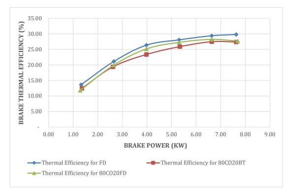
Figure 105: Brake Thermal Efficiency vs. load of CO100 and its blends.
