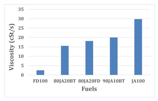
Figure 69: Viscosity of FD100 with JA100 and its blends at 40 °C.
