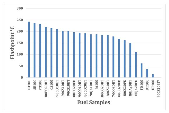
Figure 75: Flashpoint of pure plant oils -ASTM D3278.
