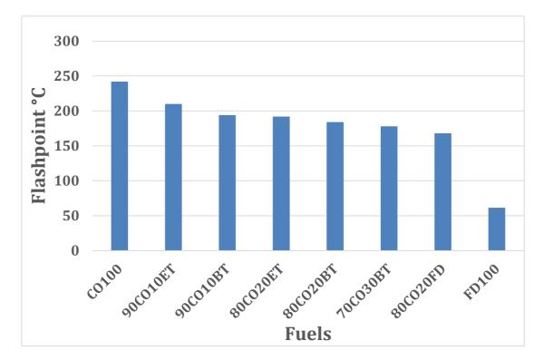
Figure 78: Flashpoint of CO100 and its blends.
