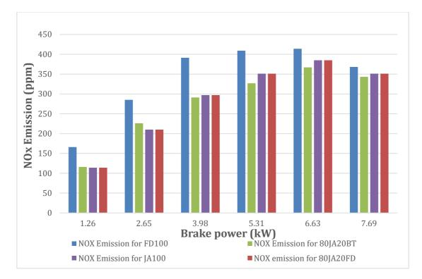
Figure 89: NO<sub>X</sub> emission vs. load of FD100, JA100 and its blends.
