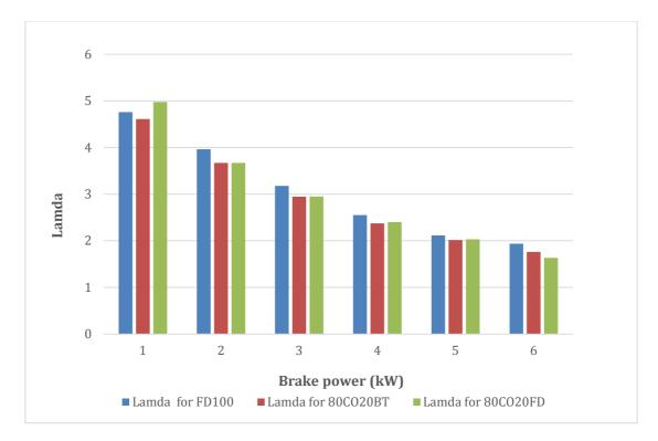
Figure 112: Lambda vs. load of FD100, CO100, and its blends.
