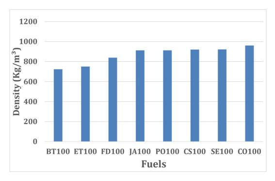
Figure 71: Density of FD100 with all pure samples.
