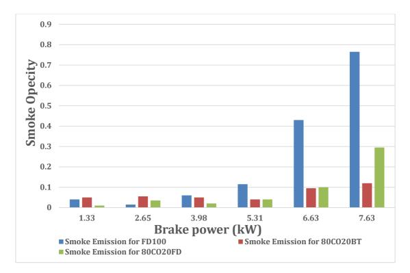
Figure 114: Smoke emission vs. load of FD100, CO100 and its blends.
