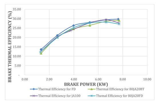
Figure 81: Brake Thermal Efficiency vs. load of JA100 and its blends.
