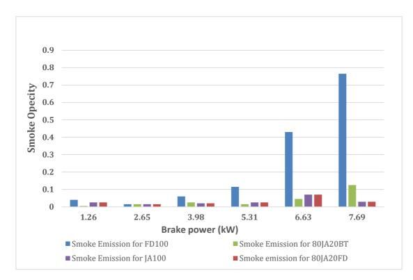
Figure 90: Smoke emission vs. load of FD100, JA100 and its blends.
