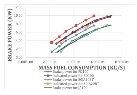
Figure 79: Brake and Indicated powers vs. Mass Fuel consumption of FD100 & JA100 and its blends.
