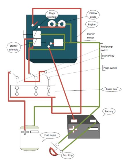
Figure 54: Engine electrical Circuit modification.
