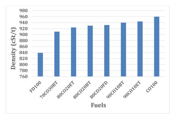
Figure 74: Density of FD100 and CO100 with its blends.
