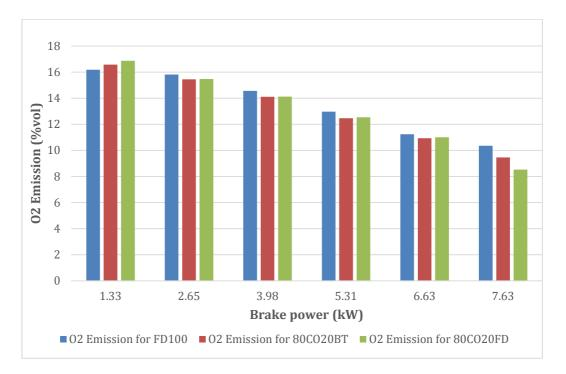
Figure 109: O2 emission vs. load of FD100, CO100 and its blends.
