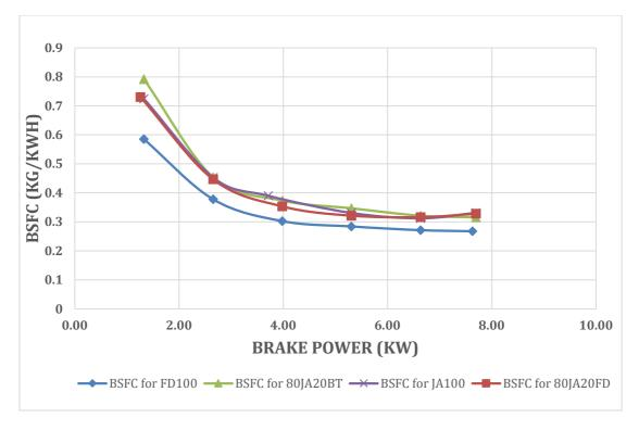
Figure 80: Brake Specific Fuel Consumption vs. load of FD100, JA100, and its blends.
