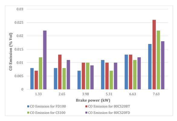
Figure 96: CO emission vs. load of FD100, CS100 and its blends.
