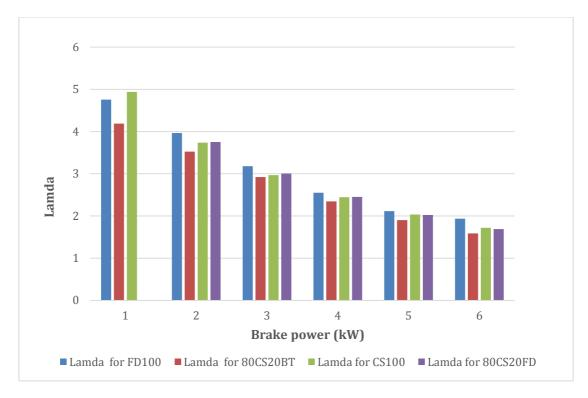
Figure 100: Lambda vs. load of FD100, CS100 and its blends.
