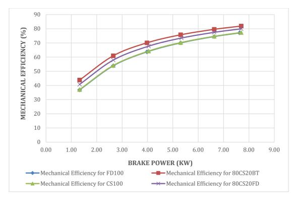
Figure 94: Mechanical Efficiency vs. load of FD100, CS100 and its blends.
