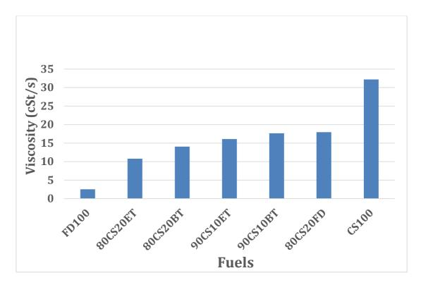
Figure 68: Viscosity of FD100 with CS100 and its blends at 40 °C.
