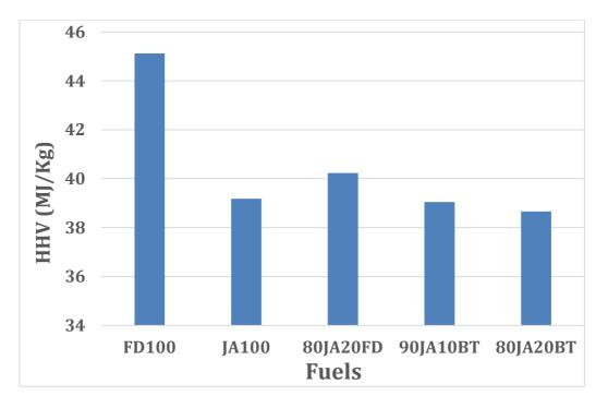
Figure 63: HHV of FD100 with JA100 with its blends.
