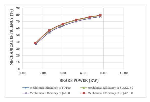
Figure 82: Mechanical Efficiency vs. load of FD100, JA100 and its blends.
