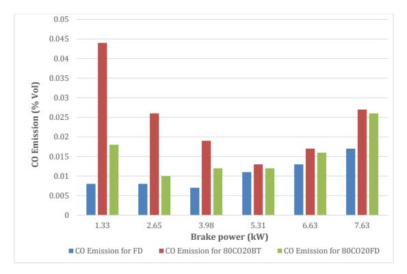
Figure 108: CO emission vs. load of FD100, CO100 and its blends.
