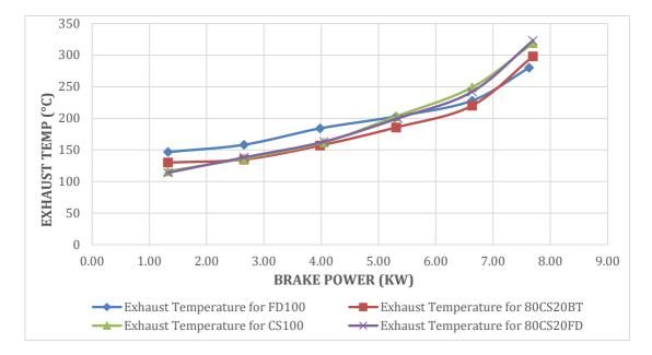
Figure 95: Exhaust temperature vs. load of FD100, CS100 and its blends.
