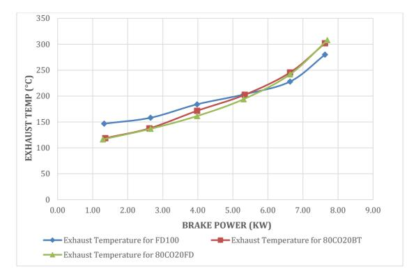
Figure 107: Exhaust temperature vs. load of FD100, CO100 and its blends.
