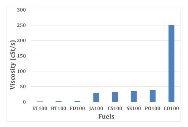
Figure 67: Viscosity of FD100 and other 100% fuels at 40 °C.
