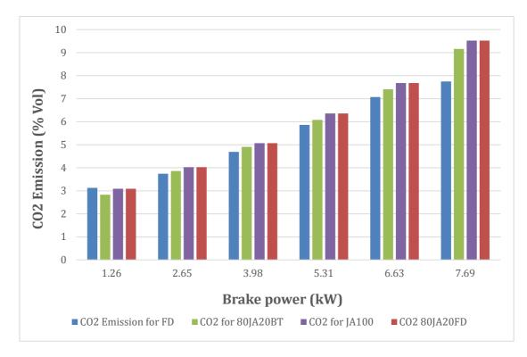
Figure 86: CO<sub>2</sub> Emission vs. load of FD100, JA100 and its blends.
