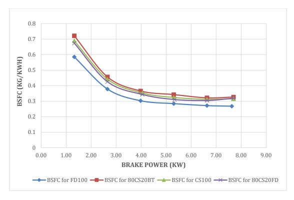
Figure 92: Brake Specific Fuel Consumption vs. load of FD100, CS100, and its blends.
