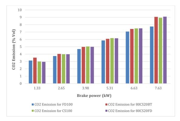
Figure 98: CO<sub>2</sub> Emission vs. load of FD100, CS100 and its blends.
