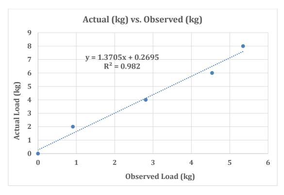
Figure 45: Froude Dynamometer Calibration.
