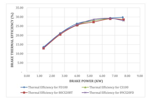
Figure 93: Brake Thermal Efficiency vs. load of CS100 and its blends.
