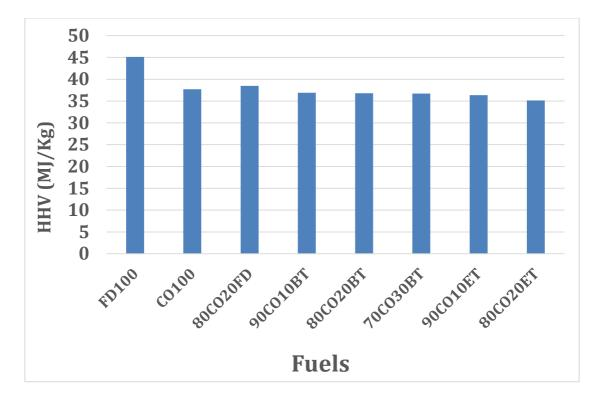
Figure 64: HHV of FD100 with CO100 and its blends.
