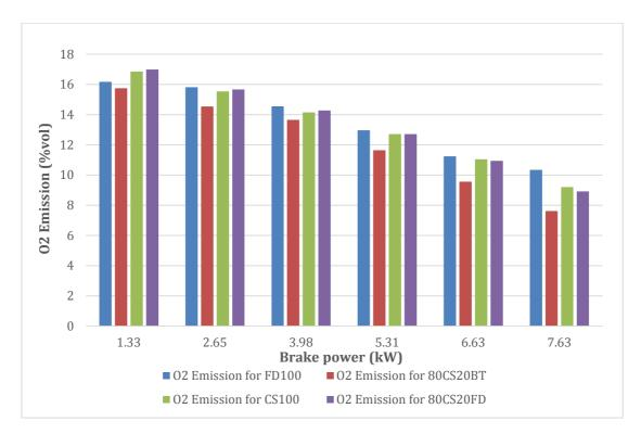
Figure 97: O<sub>2</sub> emission vs. load of FD100, CS100 and its blends.
