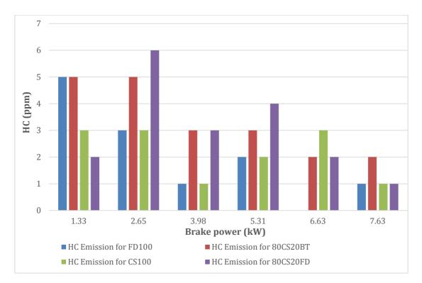
Figure 99: HC emission vs. load of FD100, CS100 and its blends.
