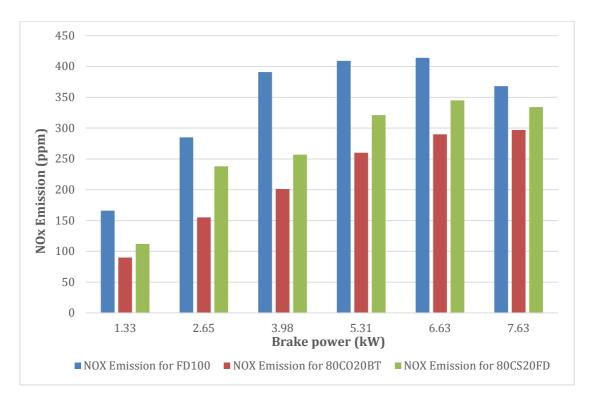
Figure 113:  $NO_X$  emission vs. load of FD100, CO100 and its blends.
