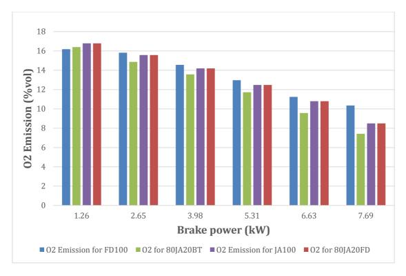
Figure 85: O<sub>2</sub> emission vs. load of FD100, JA100 and its blends.
