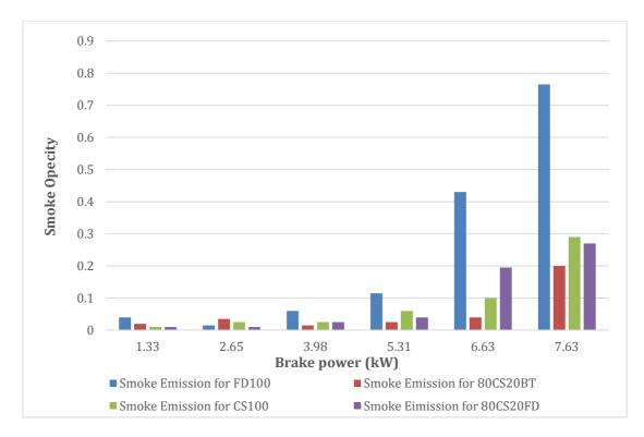
Figure 102: Smoke emission vs. load of FD100, CS100 and its blends.
