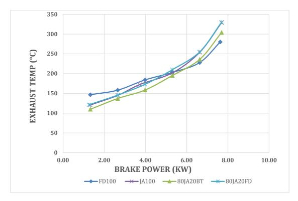
Figure 83: Exhaust temperature vs. load of FD100, JA100 and its blends.
