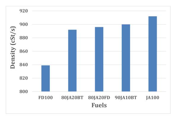
Figure 73: Density of FD100 and JA100 with its blends.
