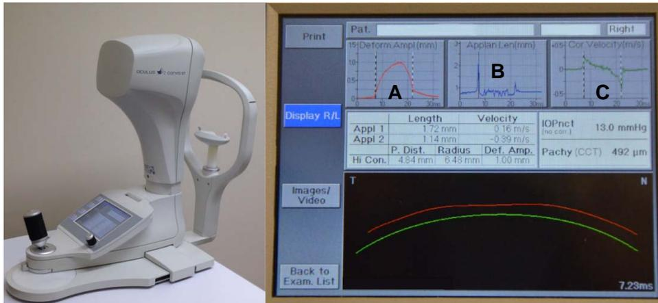
Figure 2.3 Left image: Cornea shape pre-applanation by air puff on the display screen of Corvis ST. Right image: A. First applanation of the cornea surface by air puff, B. Second applanation that resulted in further corneal deflection, C. Corneal deflection at its maximum.
