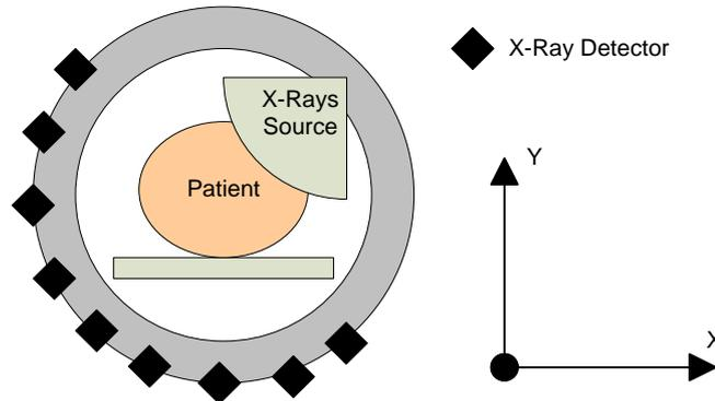
Figure 2: Diagram of a simple CT scanner.
