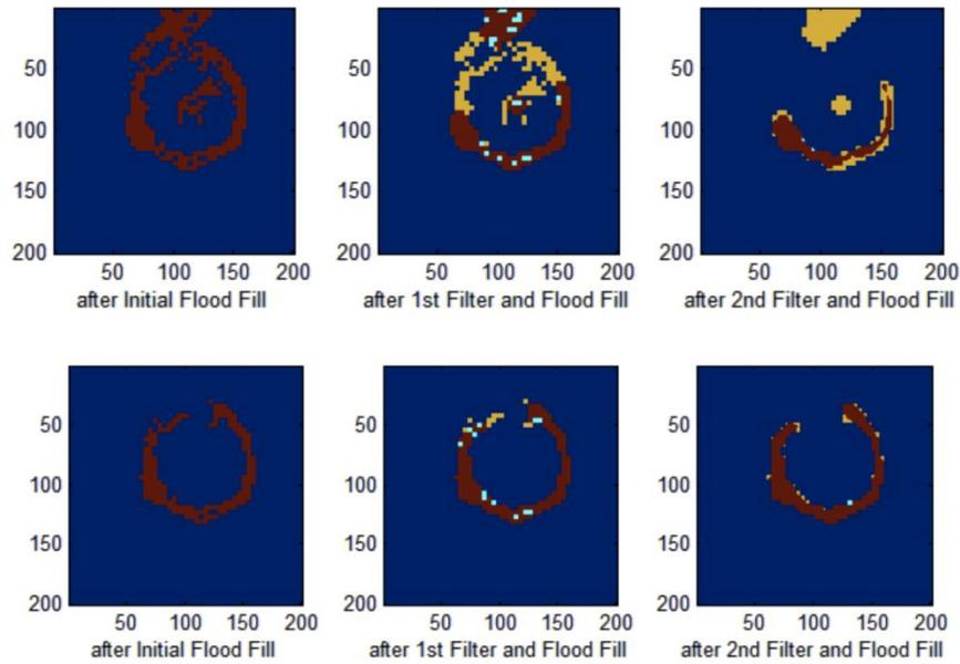
Figure 93: Using a symmetric low pass filter (top) and an asymmetric low pass filter (bottom).
