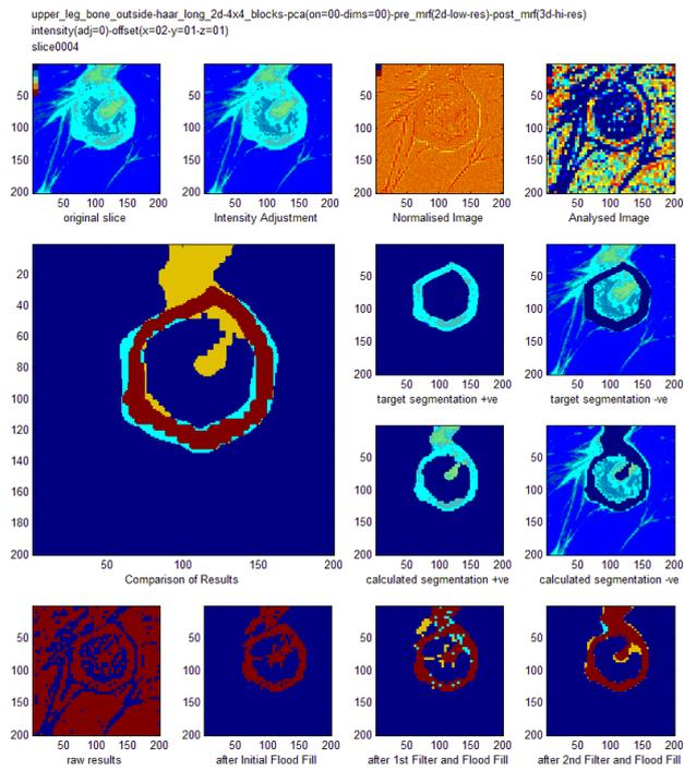
Figure 84: Segmentation performed using 2D Haar Long transforms, and using post processing as outlined in table 30.
