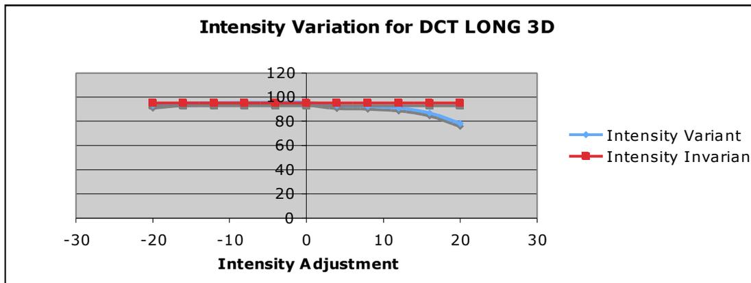
Figure 58: Plot showing the comparison of results between the Intensity Variant and Intensity Invariant methods for the DCT LONG 3D transform.
