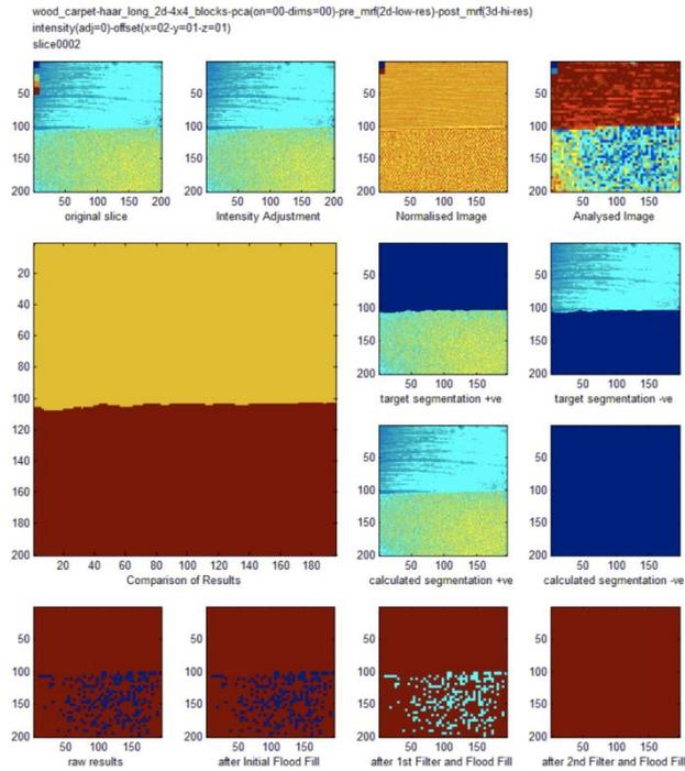
Figure 68: Example of segmentation where lack of a maximum threshold causes the segmentation to fail completely.
