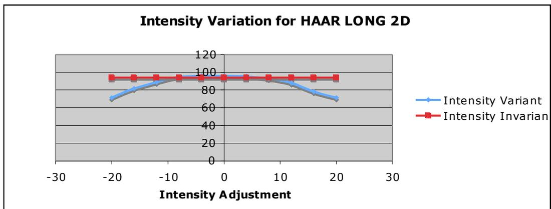
Figure 59: Plot showing the comparison of results between the Intensity Variant and Intensity Invariant methods for the HAAR LONG 2D transform.
