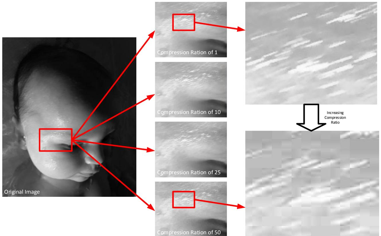
Figure 15: the effect of increasing the compression ration used when storing an image in JPEG format.
