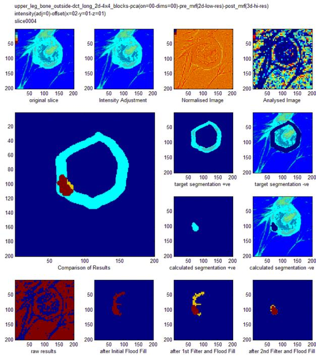
Figure 86: Segmentation preformed using 2D DCT Long transforms, and using post processing as outlined in table 30.
