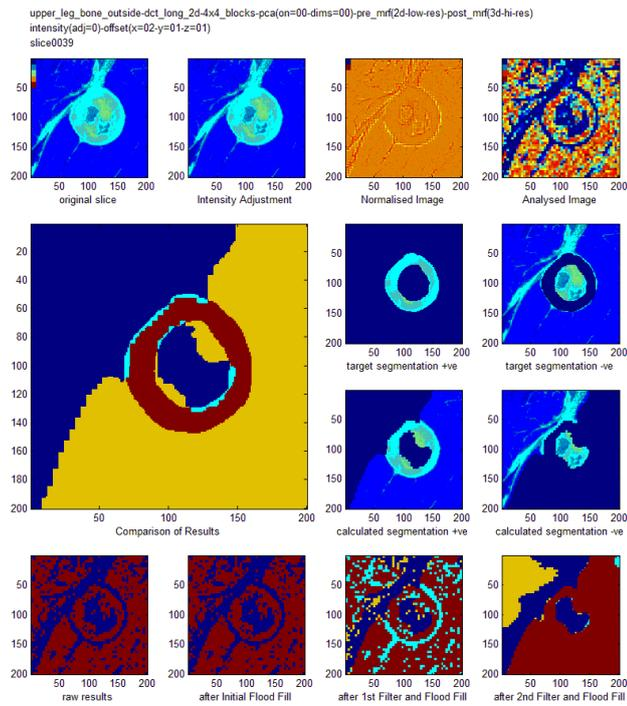
Figure 83: More complex segmentation, attempted using 2D DCT Long transforms, and post processing as described in table 28.
