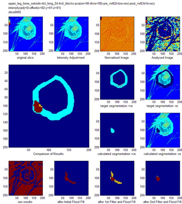
Figure 87: Segmentation preformed using 2D DCT Long transforms, and using post processing as outlined in table 30.
