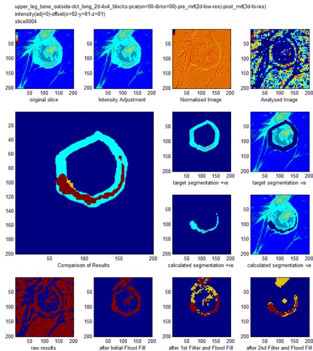
Figure 92: The initial low pass filter was responsible for over eroding the results.
