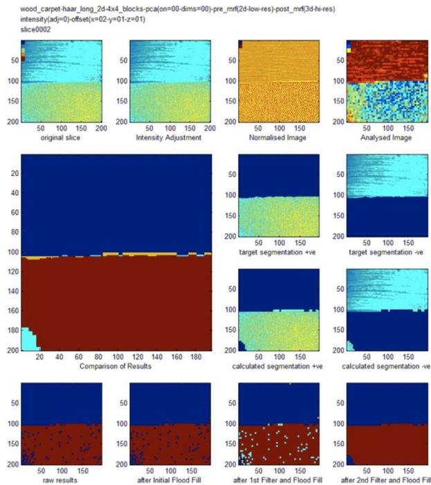
Figure 69: Example of segmentation where lack of a maximum threshold causes the segmentation to fail completely.
