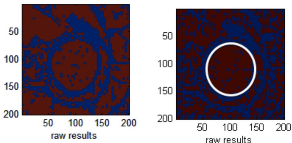
Figure 71: Left hand image shows the raw results before a maximum threshold was used. Right hand image shows the raw results once a maximum threshold has been used. The white oval annotation on the right hand image shows the approximate location of the desired segmentation.
