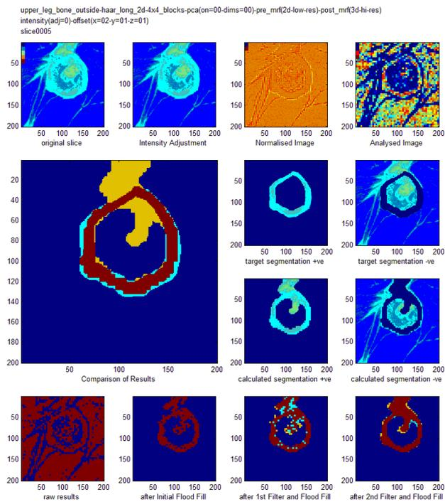
Figure 85: Segmentation performed using 2D Haar Long transforms, and using post processing as outlined in table 30.
