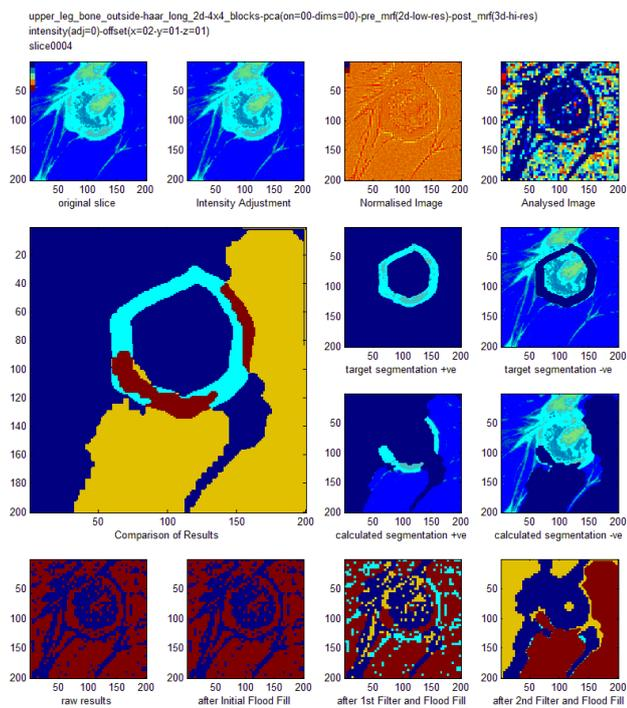
Figure 82: More complex segmentation, attempted using 2D Haar Long transforms, and post processing as described in table 28.
