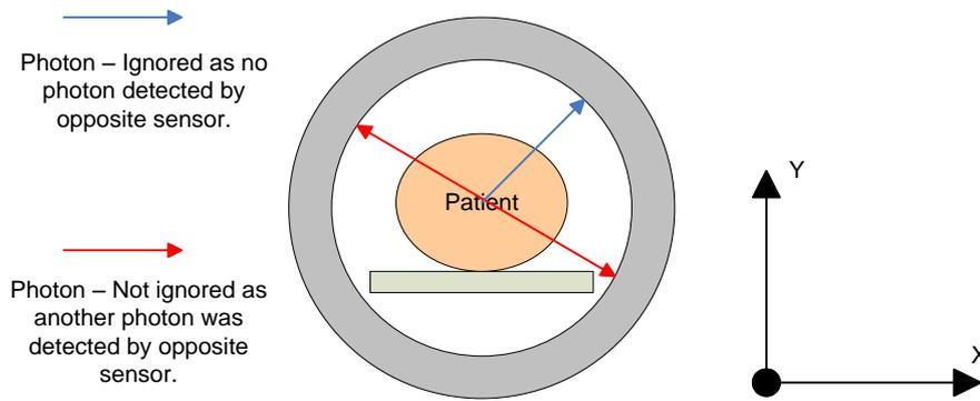
Figure 5: Photon pairs as observed by a PET scanner.
