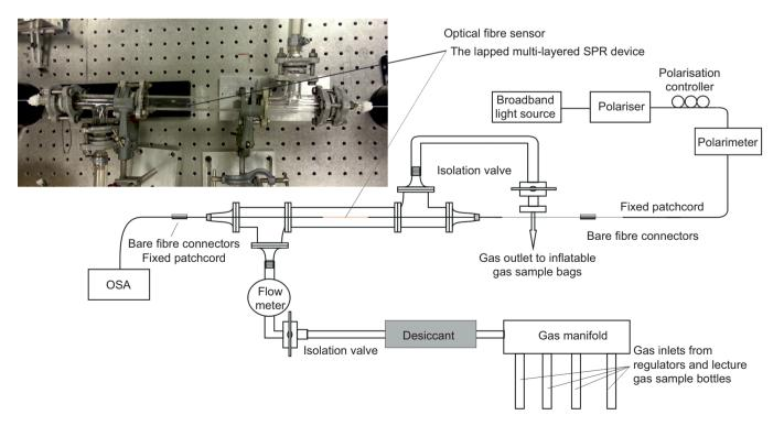
Figure 2 Scheme of gas sensing apparatus and picture of the gas chamber.
