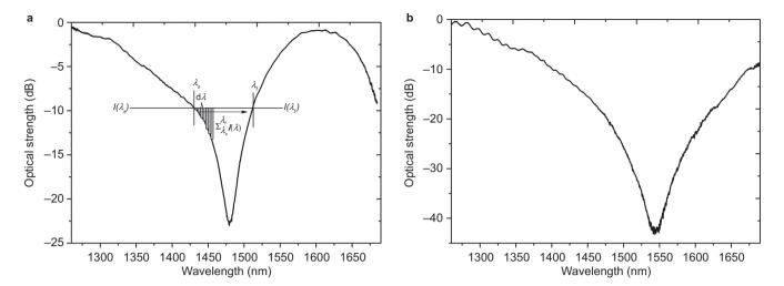
**Figure 3** (a) shows the spectral transmission feature of the LSP (UV processed with no CNTs) fiber sensor submerged in a solution with a refractive index value of 1.32 and the visualization of determining wavelength shift. (b) Shows the spectral transmission feature of the same LSP fiber sensor in **a** but with the coating of CNTs.
