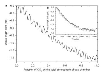
Figure 6 Typical spectral behavior of the fiber sensor with an LSP wavelength resonance at 1390 nm, (a) as a function of the fraction of CO2 in the surrounding atmosphere (b) showing the spectral response of the sensor with respect to the time taken for the experiment to be completed
