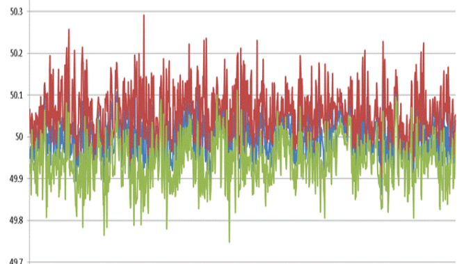
Fig. 15. Typical plot of frequency variation with time over a week, showing maximum, minimum and mean values of frequency over each time segment and the frequency excursions (spikes over 50.2Hz and under 49.8Hz)
