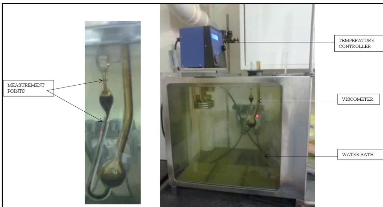
**Figure 3.2:** Experimental setup for viscosity measurement
