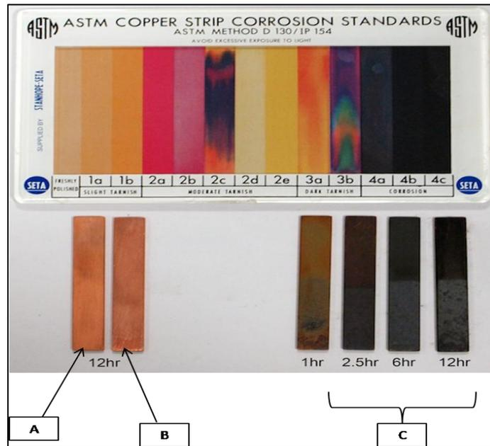
**Figure 5.5:** Copper strip corrosion results shown for biodiesel [A], diesel [B] and sewage sludge pyrolysis oil [C]
