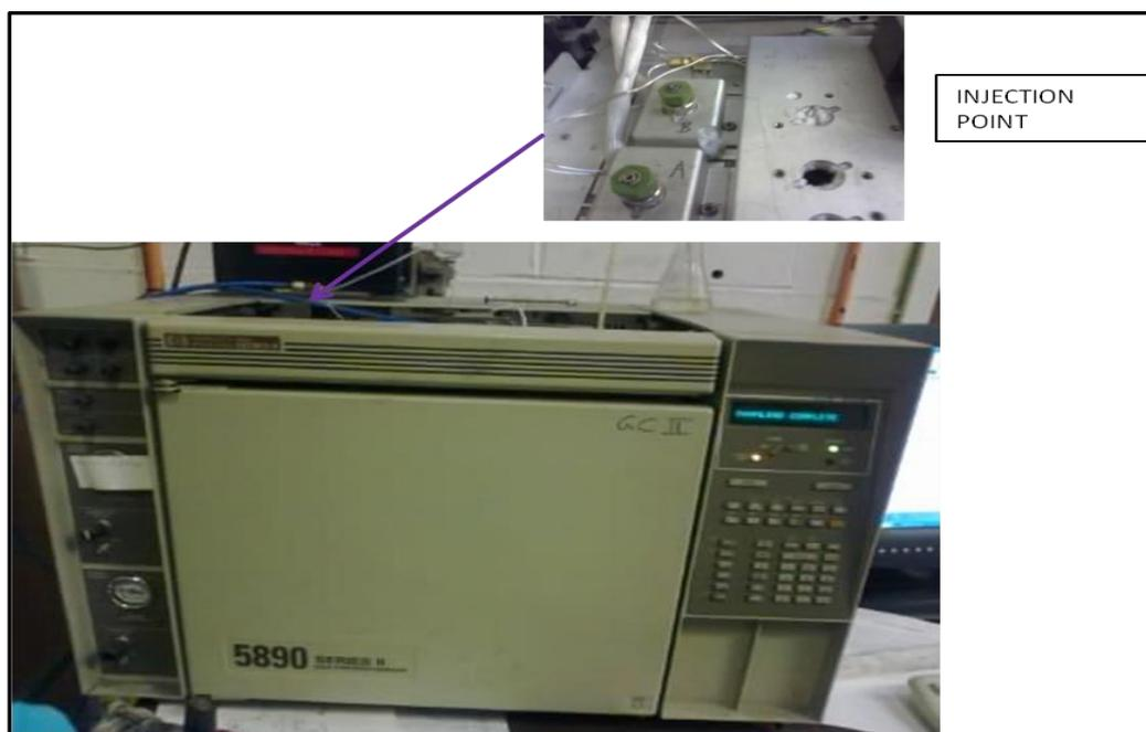
**Figure 3.8:** Gas chromatograph for permanent gas measurements
