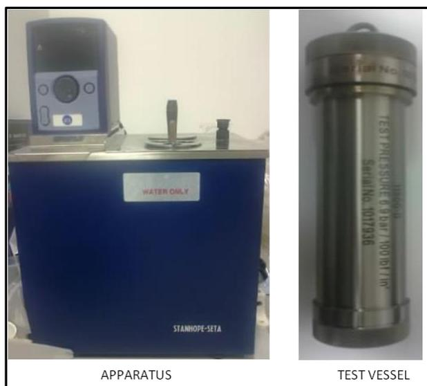
**Figure 3.4:** The Stanhope Seta equipment for the copper corrosion test
