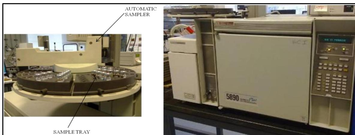
**Figure 3.1:** The gas chromatograph mass spectrometry 5890 series
