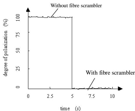
Fig. 6. Reduction of polarisation degree for eliminating the effect of polarisation fading
