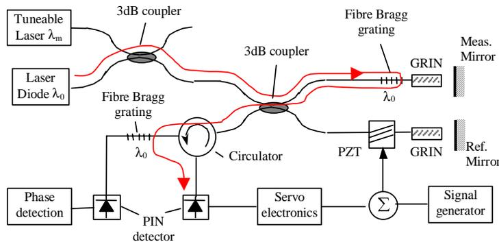
Fig. 1. The schematic of multiplexed fibre interferometer
