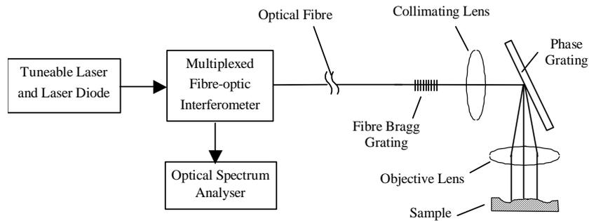
Fig. 2. The schematic of on-line surface measurement by means of MFI
