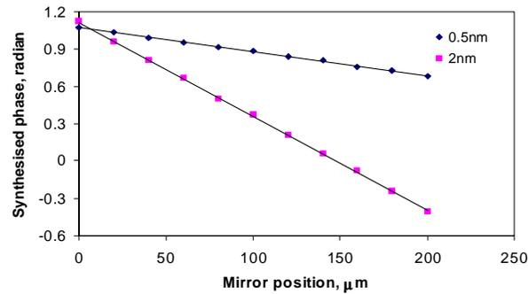
Fig. 4. Experimental results of ADM by synthesised phase over 200 $\mu\text{m}$  measurement range
