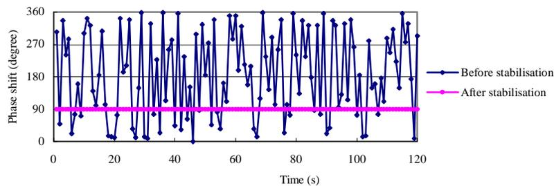
Fig. 3. The phase shift of fibre interferometer before and after stabilization
