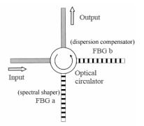
Fig. 1. Architecture of the system. Input signal is processed by two oppositely chirped FBGs, which are connected by an optical circulator.
