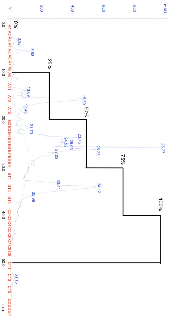
**Figure 7.4.2. HPLC separation of an aqueous extract of *Fagonia cretica*.** Following aqueous extract purification by SPE, the eluate was subjected to HPLC on a C18 column. This figure is typical of chromatograms observed using detection at 280nm. X axis - retention time, Y-axis - relative absorbance units (UV detection: 254nm). Black lines represent percentage of methanol in mobile phase.
