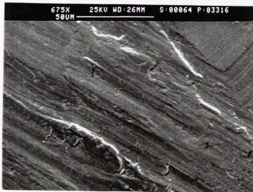
Figure 7.22 13 mm diameter M2 HSS slow helix drill, cutting speed 490 rpm.
