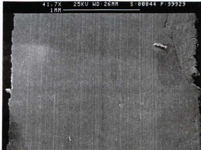
Figure 6.36 M2 HSS, cutting speed 40 m/min, rake angle 6°, flank angle 5°, and feed rate 0.15 mm/rev.
