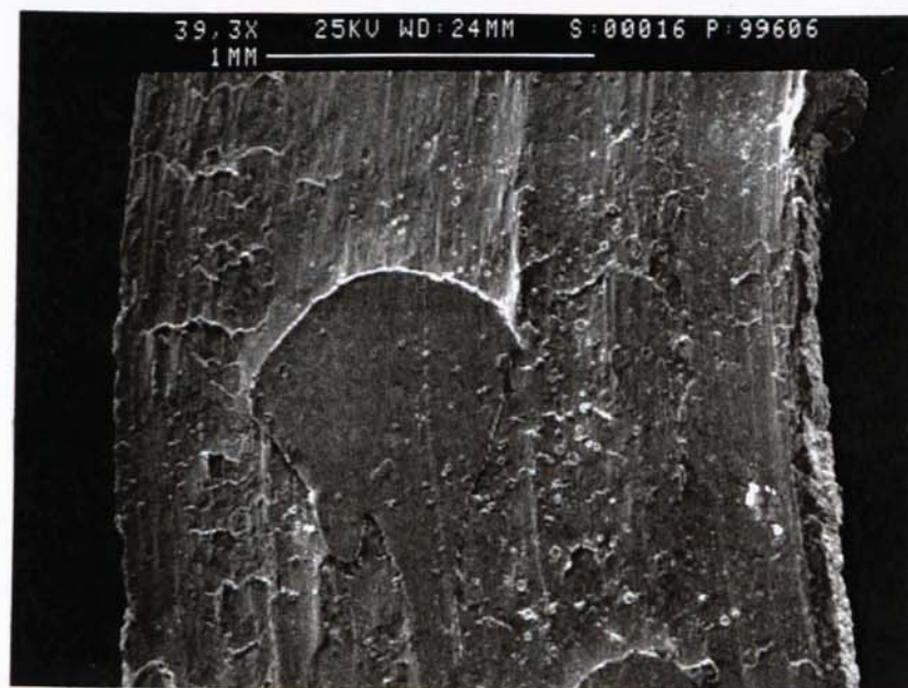
Figure 6.35 M2 HSS, cutting speed 30 m/min, rake angle 6°, flank angle 5°, and feed rate 0.15 mm/rev.
