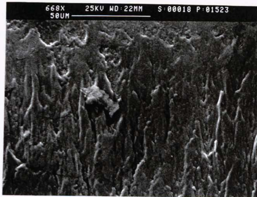
Figure 6.40 M2 HSS, cutting speed 20 m/min, rake angle 10°, flank angle 10°, and feed rate 0.15 mm/rev.
