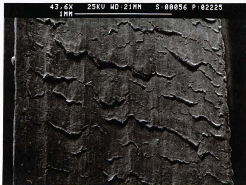
Figure 7.18 13 mm diameter M2 HSS standard helix drill, cutting speed 244 rpm.
