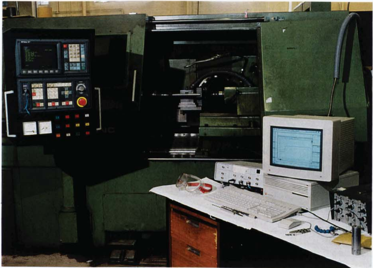
Figure 4.4 Photograph of Torshalla CNC lathe with force equipment
