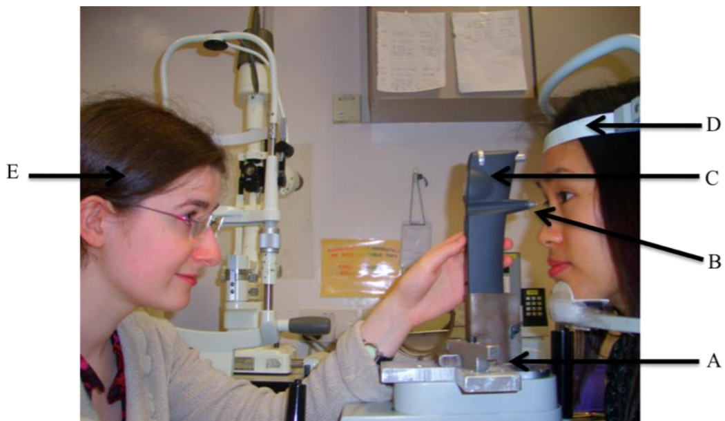
Figure 8.1 iCare tonometry experimental setup side view. A: Custom-designed housing for the iCare tonometer, B: Graticule for estimating location of scleral measurement, C: iCare tonometer, D: Head rest for subject, E: Examiner ED.
