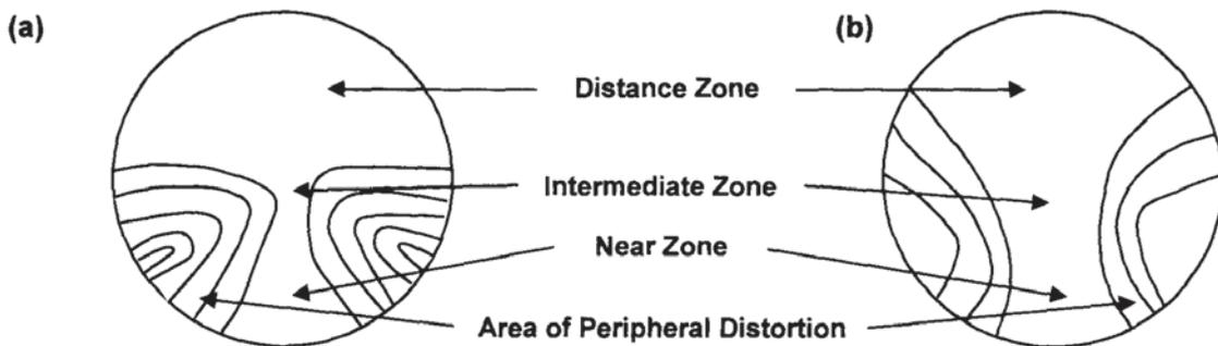
**Figure 1.5 Astigmatism plots displaying the type of progression expected of (a) Varilux 1 lens and (b) Varilux 2 lens – reproduced and modified from Meister and Fisher (2008)**
