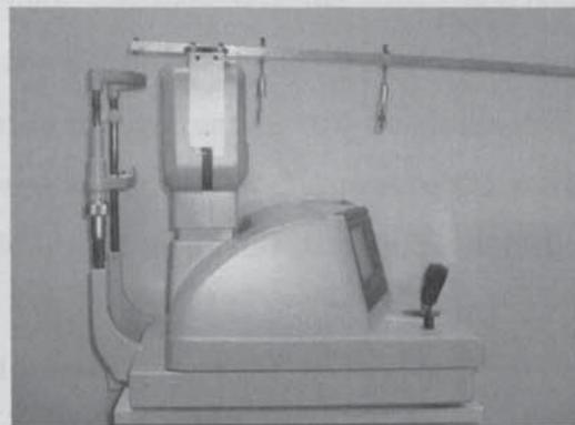
**Figure 3.2** The Shin-Nippon SRW-500 autorefractor (Ajinomoto Trading Inc., Tokyo, Japan) with Badal optometer attachment – photographed at the Aston University Optometry Clinic
