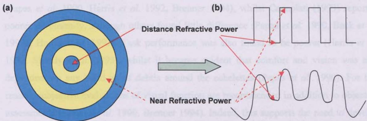
**Figure 1.10 (a) Design of the Acuvue™ bifocal contact lens, and (b) the intended (top) and actual (bottom) power profiles – produced based on a figure in Hough (2002)**
