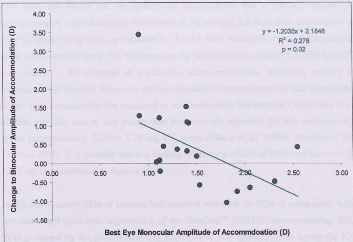
**Figure 7.7 Predictive changes in the subjective amplitude of accommodation from unilateral (best eye) to bilateral implantation of the Tetraflex™ KH3500 ‘accommodating’ IOL (n=19 subjects)**
