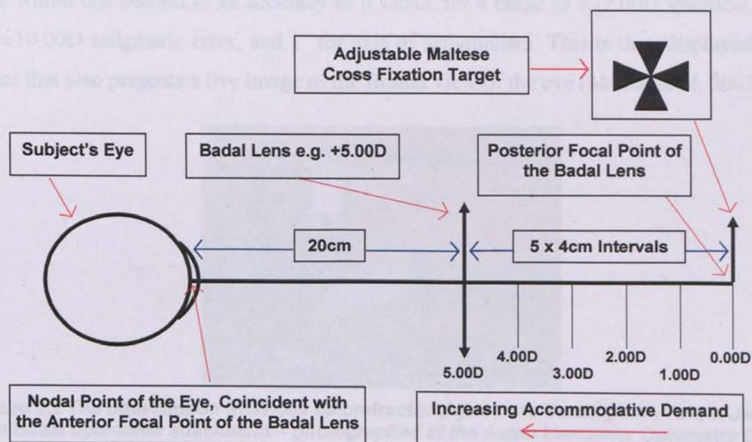
Figure 3.1 Objective measurement of the amplitude of accommodation (AoA) with an optometer and a Badal system – produced based on the equipment shown in Figure 3.2
