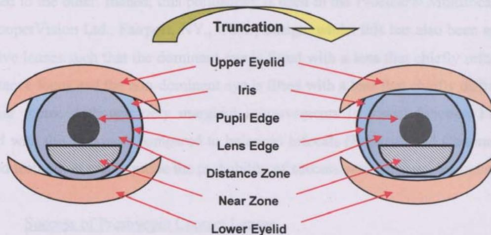
**Figure 1.11 Lens truncation creates flat top and bottom edges so that the eyelids can act to prevent lens rotation – produced based on a description in Borish and Soni (1982)**
