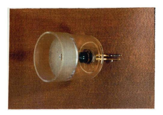
Figure A2.3 Colour print of an angled view of the FE "cup", without the "lid" in place. The metal disc with artificial pupil and central (flickering) LED can be identified. This photograph was taken before the FE was sprayed and the diffusing sheets were added.
