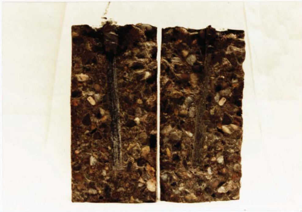
Figure 6.8 OPENED SPECIMEN CONTAINING STEEL WITH 'SULPHATE RUST' (84 WEEKS)
