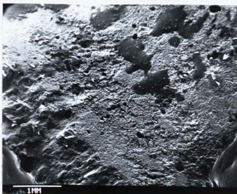
Figure 6.11 INTERFACIAL LAYER FORMED AGAINST 'SULPHATE RUST' (x 20)
