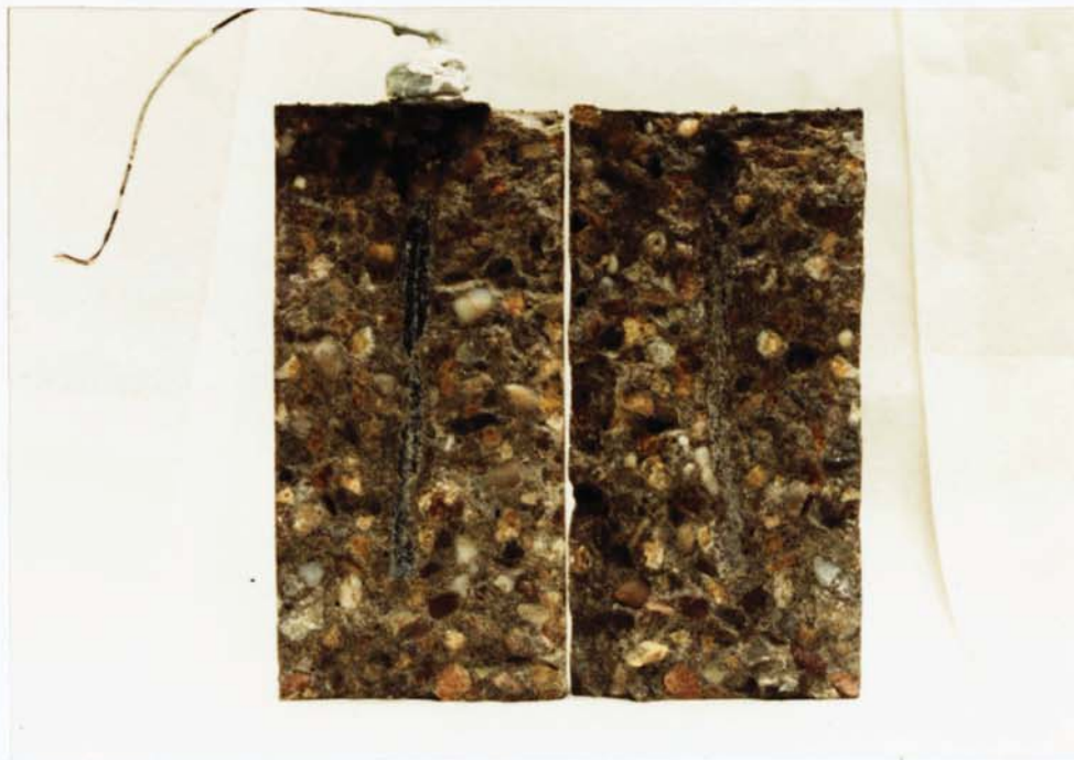
Figure 6.6 OPENED SPECIMEN CONTAINING STEEL WITH 'WATER VAPOUR RUST' (84 WEEKS)
