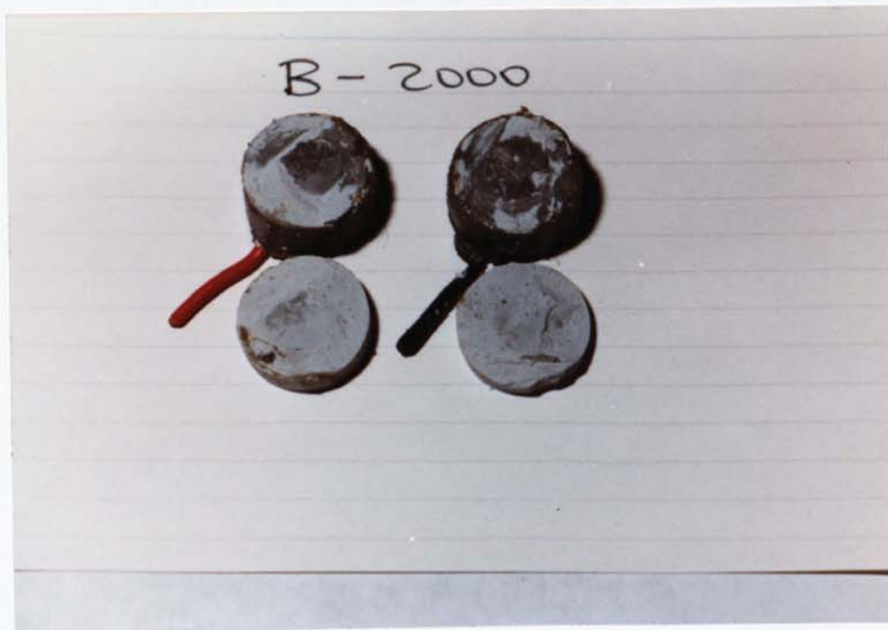
Figure 5.17 MILD STEEL IN ALITE CONTAINING 2000 ppm \text{Cl}^- (10 WEEKS)
