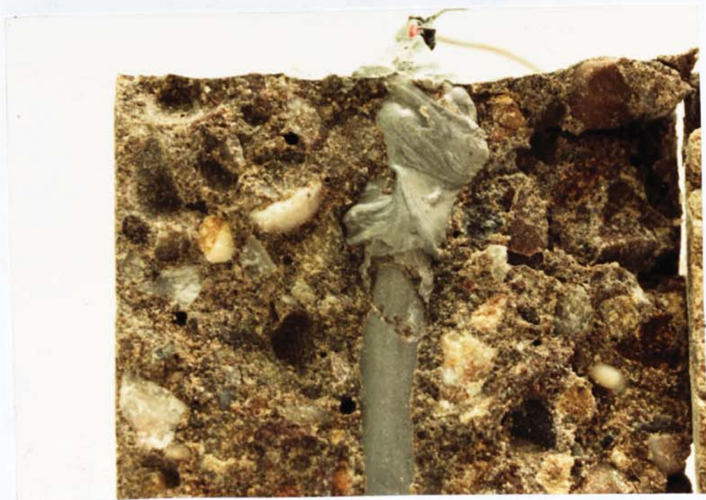
Figure 6.13 SMALL AREA OF CORROSION ON EMBEDDED CLEAN STEEL BAR EXPOSED TO A CHLORIDE ENVIRONMENT (84 WEEKS)
