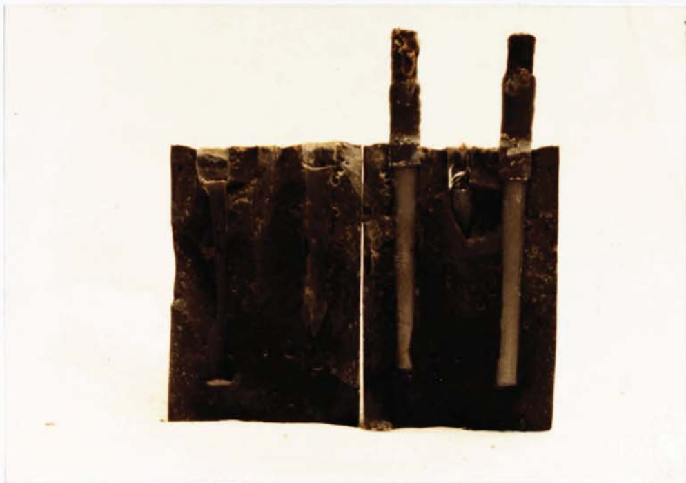
Figure 7.9 EMBEDDED STEEL SPECIMEN SHOWING NO CREVICE ATTACK (1.84% sodium nitrite, plus 2% sodium benzoate, plus 2% \text{Cl}^- , 30 weeks)
