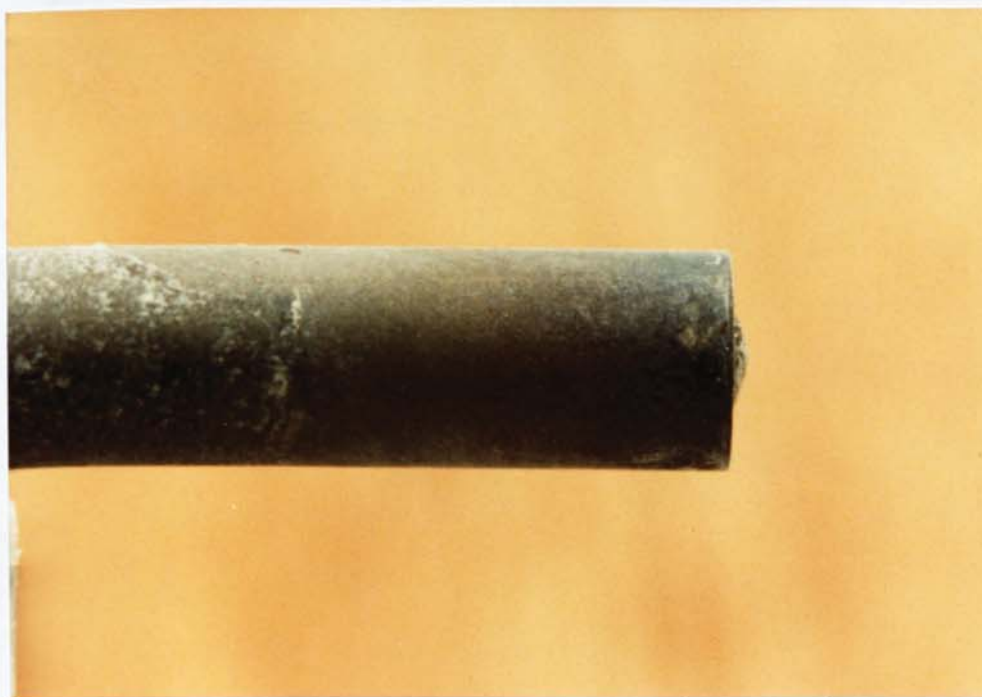
Figure 6.14 APPEARANCE OF STEEL BENEATH MASKING (84 WEEKS)
