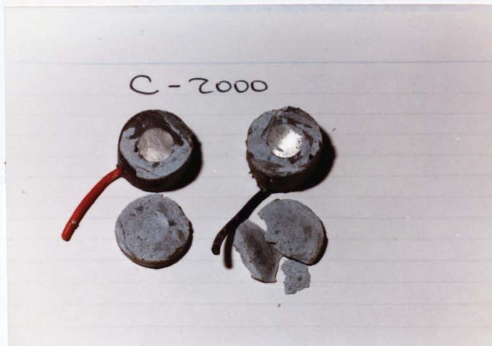
Figure 5.18 MILD STEEL IN ALITE, IN CALCIUM HYDROXIDE SOLUTION CONTAINING 2000 ppm \text{Cl}^- (10 WEEKS)
