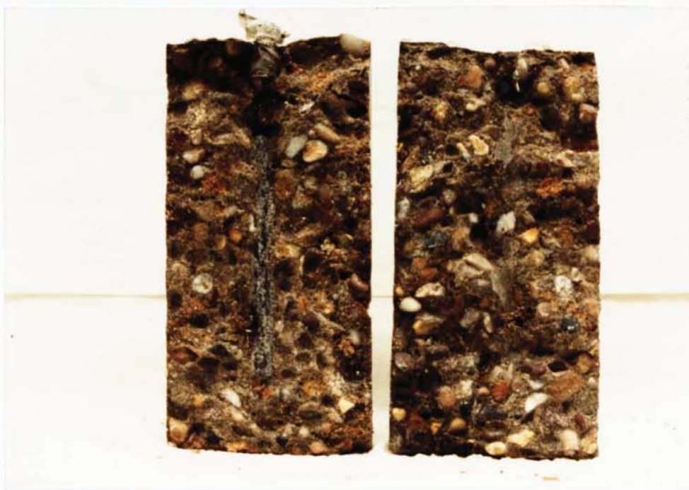
Figure 6.7 OPENED SPECIMEN CONTAINING STEEL WITH 'CHLORIDE RUST' (84 WEEKS)
