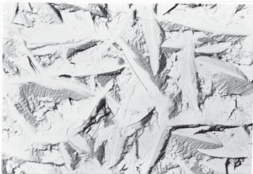
Fig.(72) Surface topography X 8.4k for 10 minutes deposit using air agitation, solution containing 110 g/l \text{CoSO}_4 \cdot 7\text{H}_2\text{O} .
