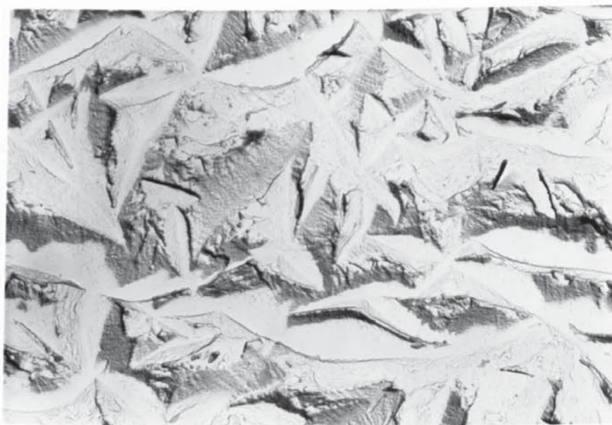
Fig.(73) Surface topography X 8.4k for 15 minutes deposit using air agitation, solution containing 110 g/l \text{CoSO}_4 \cdot 7\text{H}_2\text{O} .
