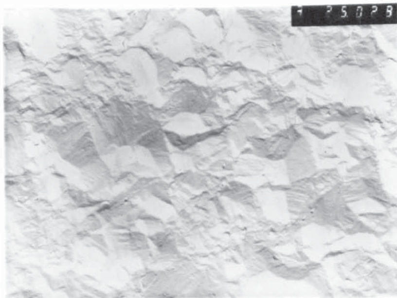
Fig.(69) Surface topography X 8.4k for 15 minutes deposit using ultrasonic agitation 350 watts.
