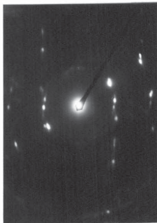
D Diffraction pattern of a large grain shown in Fig.(34) C
