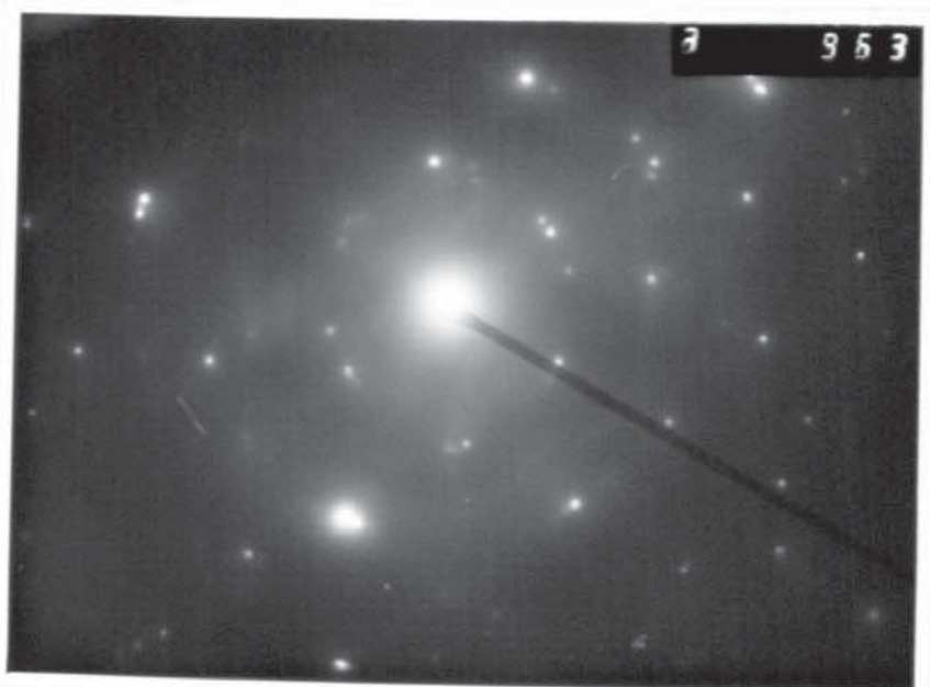
C Diffraction pattern of a grain shown in Fig. (24)B
