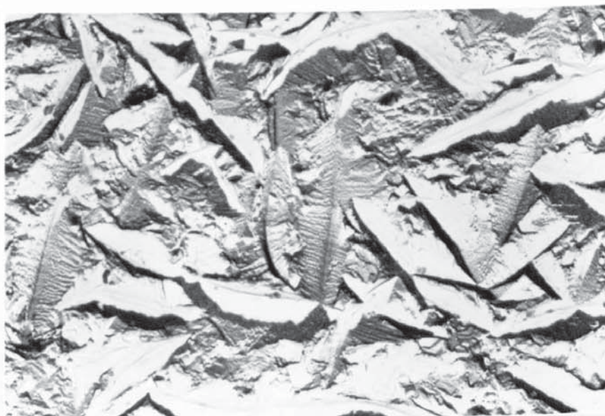
Fig.(71) Surface topography X 8.4k for 5 minutes deposit using air agitation, solution containing 110 g/l \text{CoSO}_4 \cdot 7\text{H}_2\text{O} .
