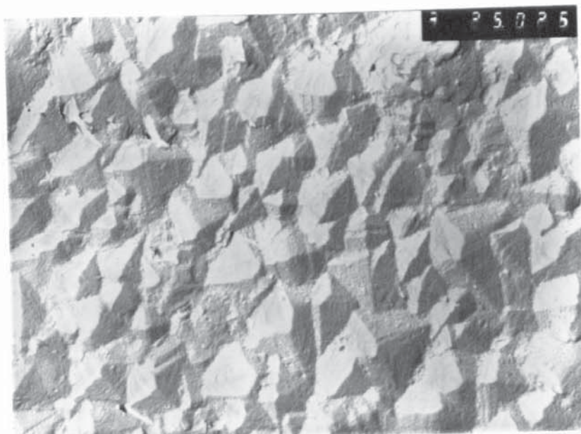
Fig.(65) Surface topography x 8.4k for 15 minutes deposit using air agitation.
