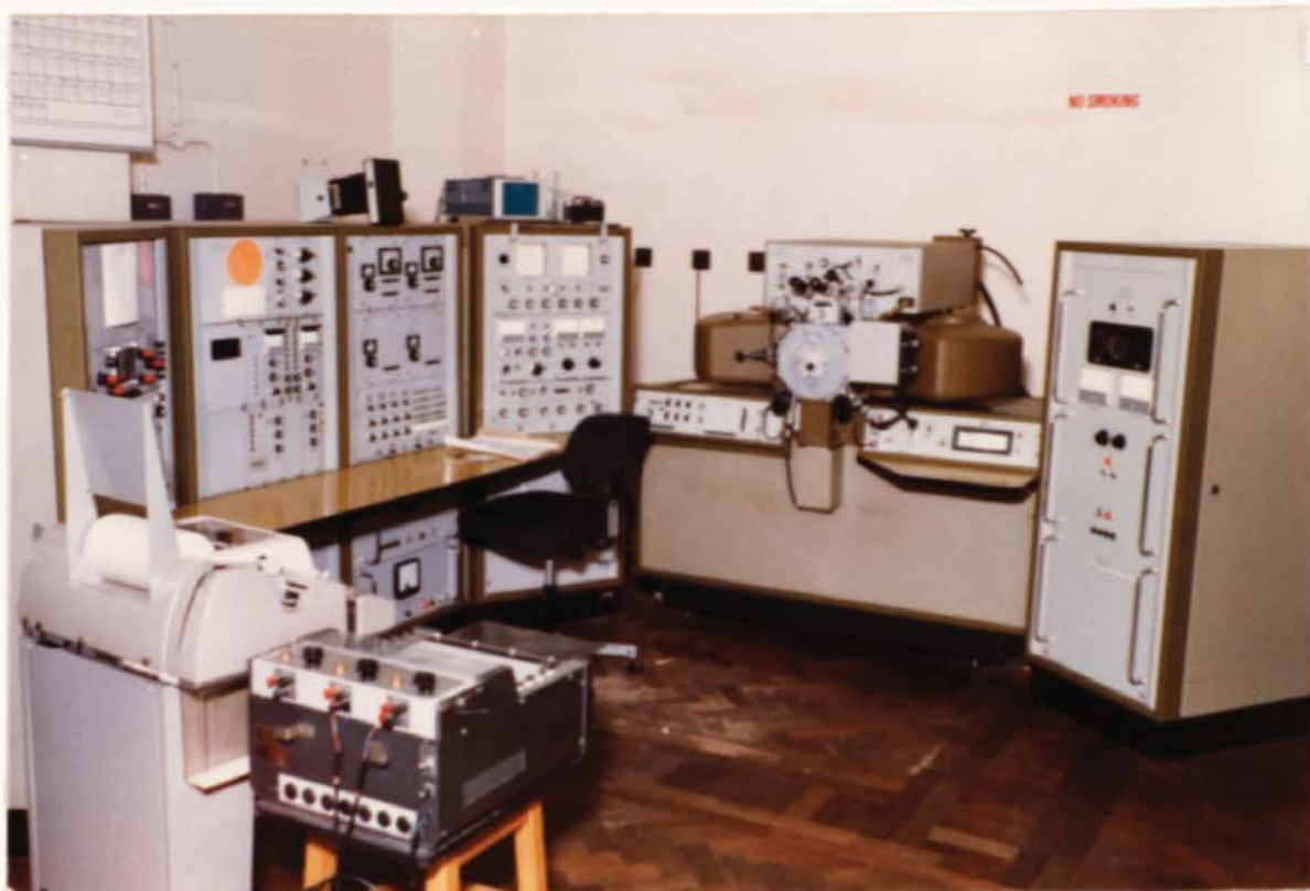
Fig.(11) Electron Probe Microanalyser Model Cambridge Microscan V.
