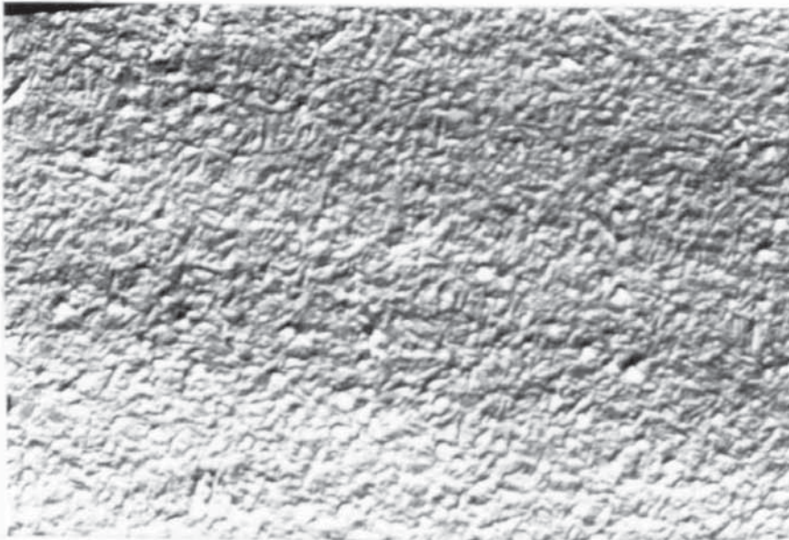
Fig.(74) Surface topography X 8.4k for 1 minute deposit using ultrasonic agitation 350 watts, solution containing 110 g/l \text{CoSO}_4 \cdot 7\text{H}_2\text{O} .
