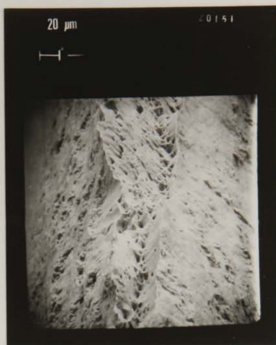
(b) Unirradiated, \sigma_{\text{Nett}} = 107.2 \text{ MNm}^{-2}
