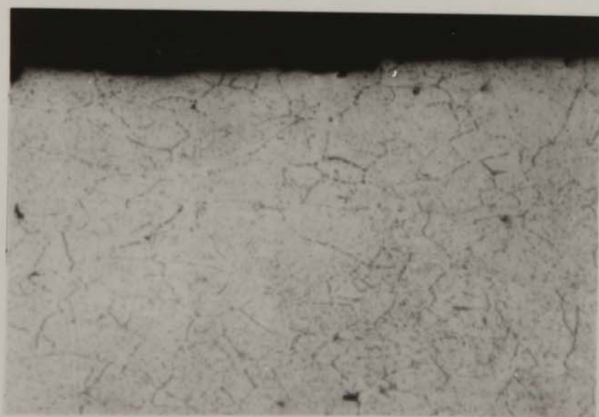
FIG 46 Surface cracks in gauge length of specimens tested in (a) iodine vapour (b) air (c) vacuum at 80\text{MNm}^{-2} and 750^{\circ}\text{C} Stress axis horizontal Magnification X 200
