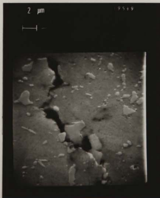
FIG 42 Creep crack growth in type 316 steel at 750°C
