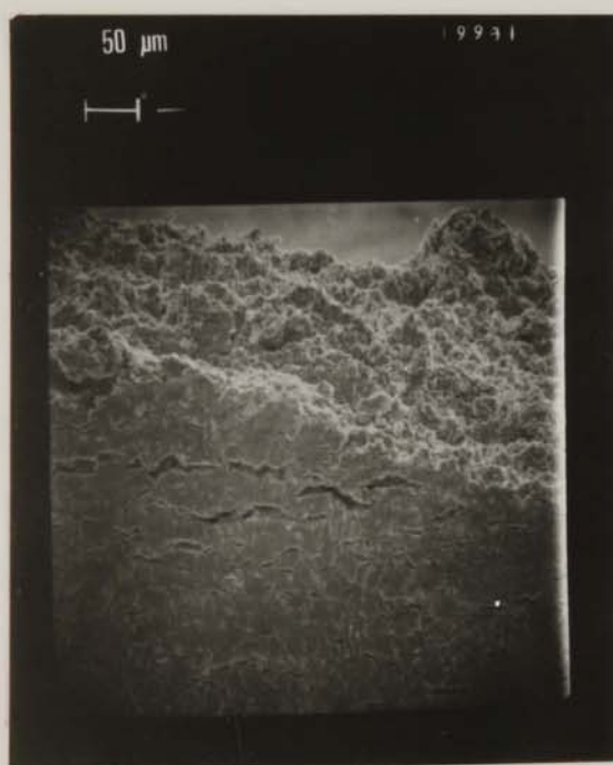
(c) Irradiated, \sigma_{\text{Nett}} = 65.8 \text{ MNm}^{-2}
