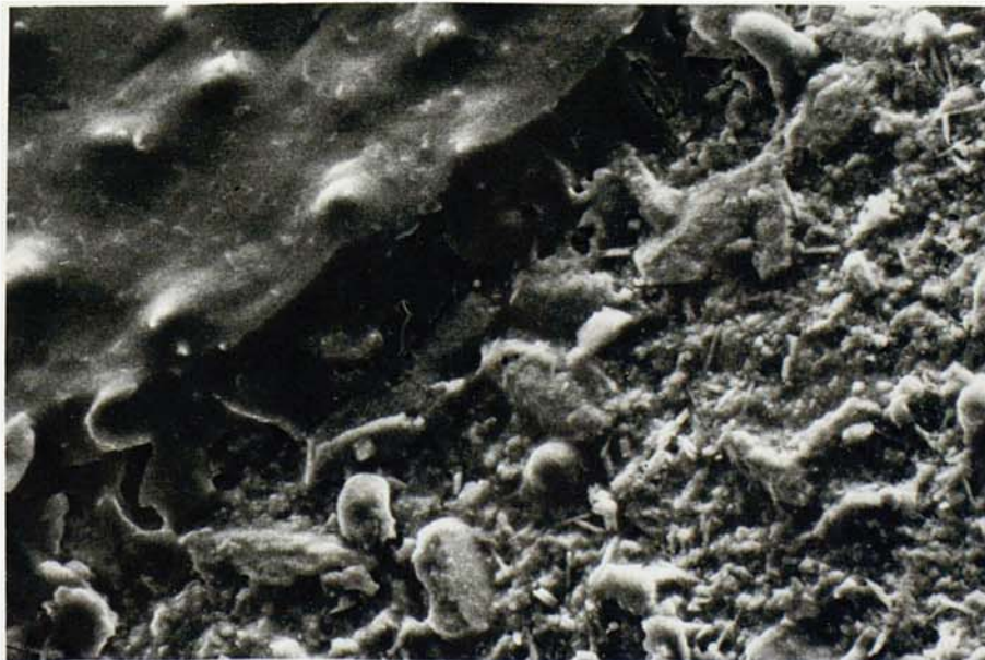
0.6 W/C ratio 28 day cure cement adhesion surface showing epoxy 'scales' adhering (SEM). Note also possible lack of wetting over rest of surface. Horizontal dimension = 5 mm.
