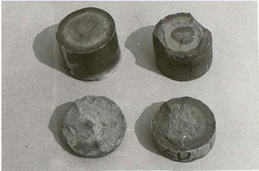
FIGURE 8.2a CEMENT CYLINDERS IMPREGNATED WITH PMMA
