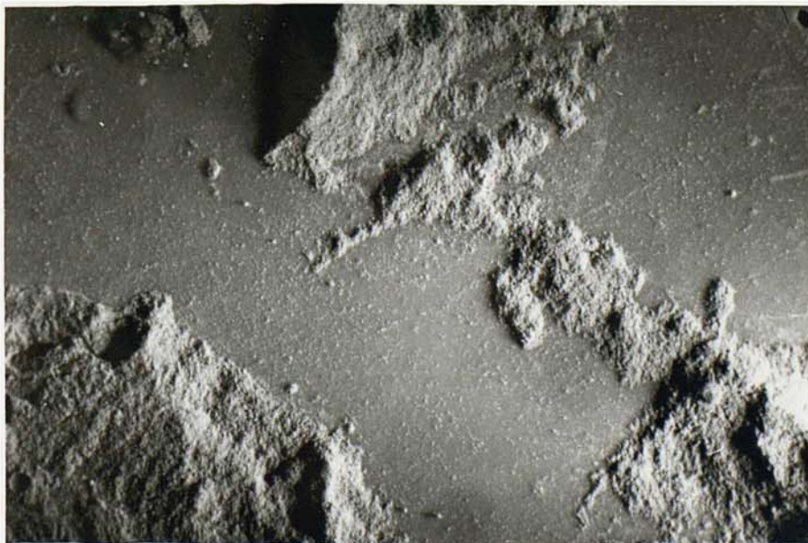
FIGURE 4.11b SINGLE-INTERFACE SPECIMENS WITH LOCUS OF FAILURE PASSING FROM INTERFACE TO CEMENT
