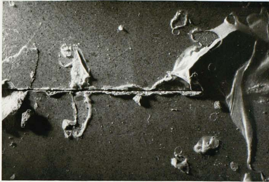
FIGURE 4.14c LOCUS OF FAILURE IN EVE-O-STICK
