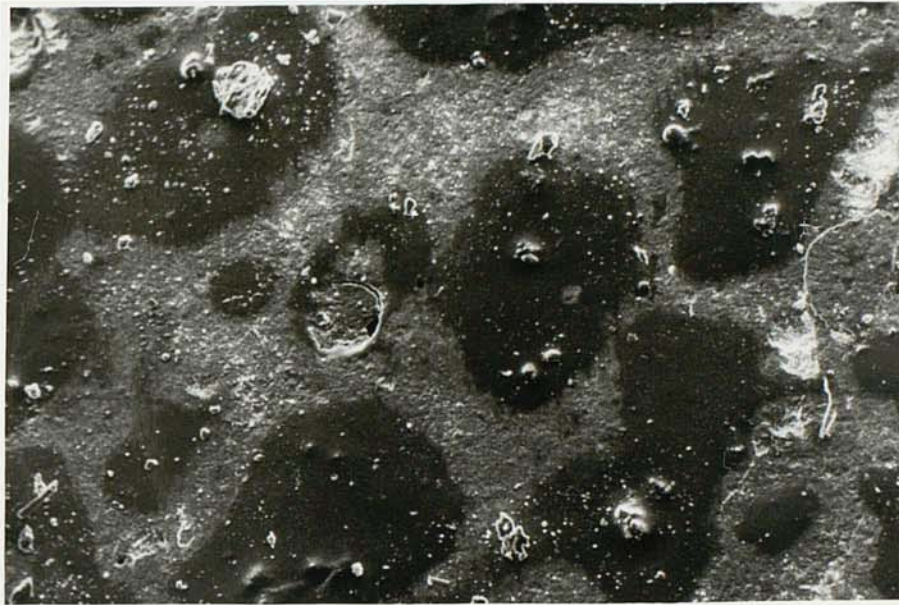
0.5 W/C ratio 28 day cure cement adhesion surface (SEM). Horizontal dimension = 5 mm.
