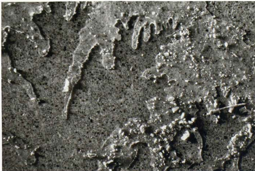
FIGURE 4.14b LOCUS OF FAILURE IN POLYSTYRENE
