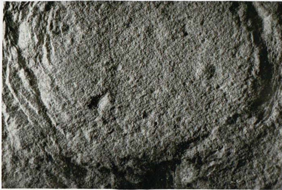
FIGURE 4.8 RING STRUCTURE ON DOUBLE-INTERFACE SHEAR SPECIMEN
