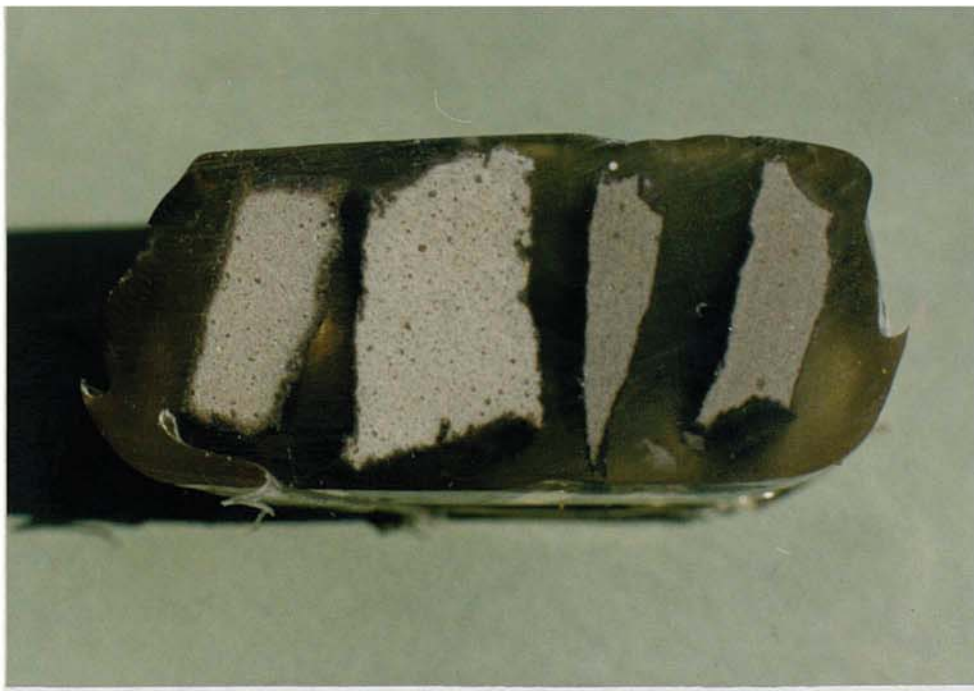
FIGURE 6.2 POLISHED SURFACE OF CEMENT / EPOXY RESIN
