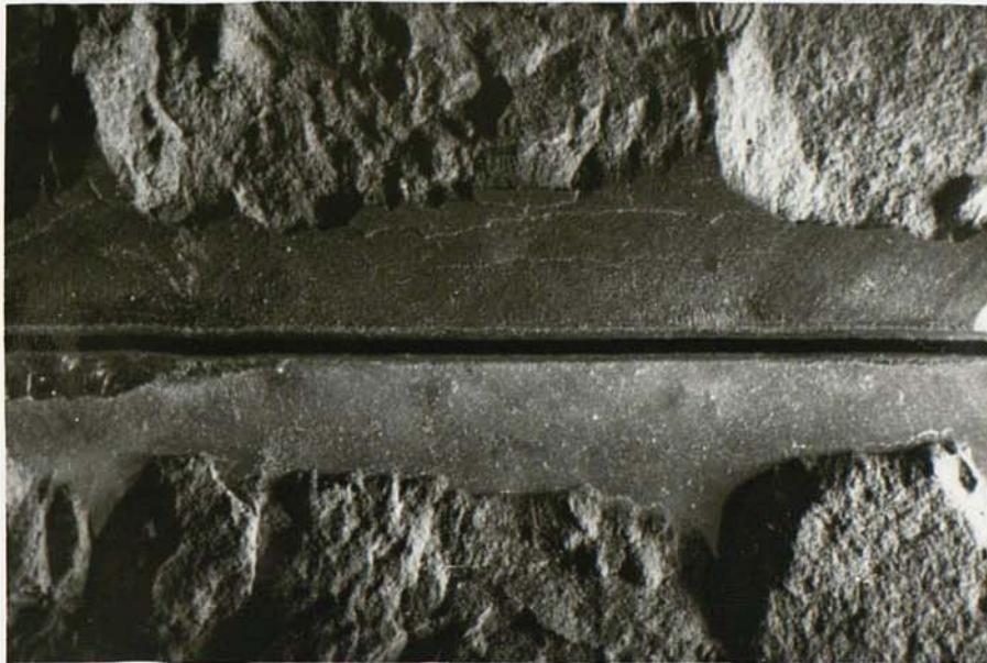
FIGURE 4.12a LOCUS OF FAILURE OF SINGLE-INTERFACE SPECIMENS USING EPOXY RESIN
