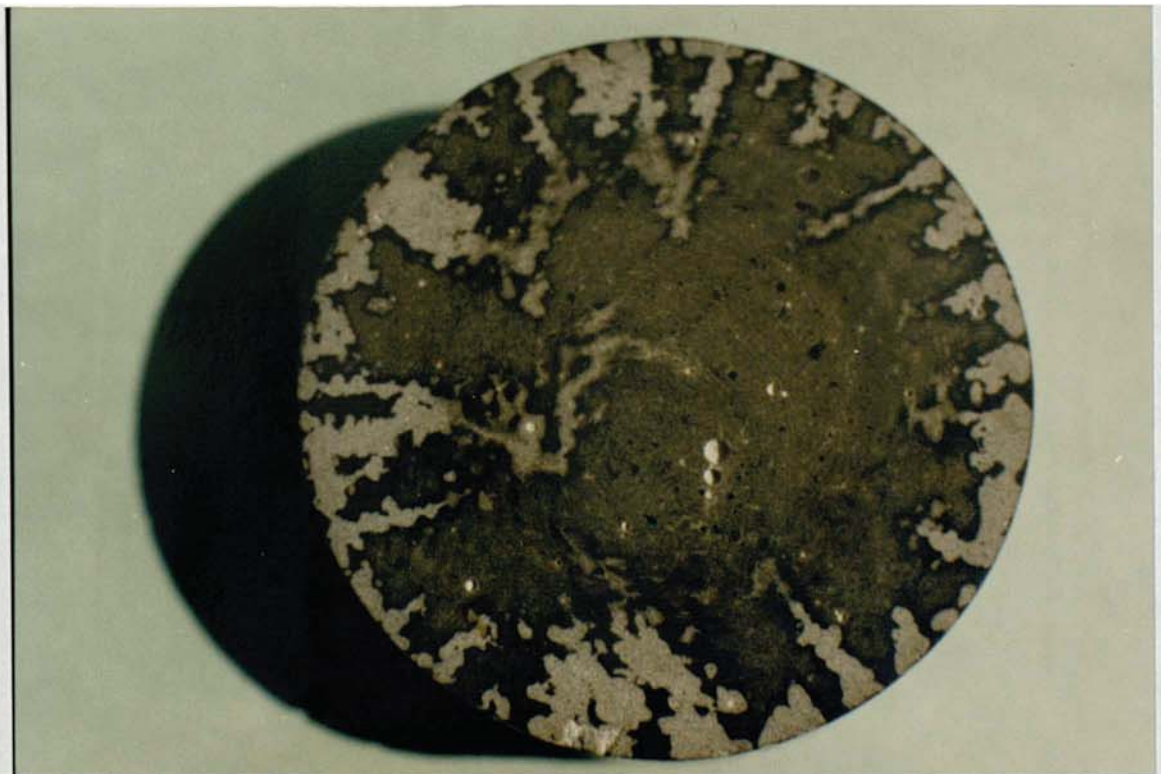
FIGURE 8.2b CEMENT CYLINDERS IMPREGNATED WITH PMMA
