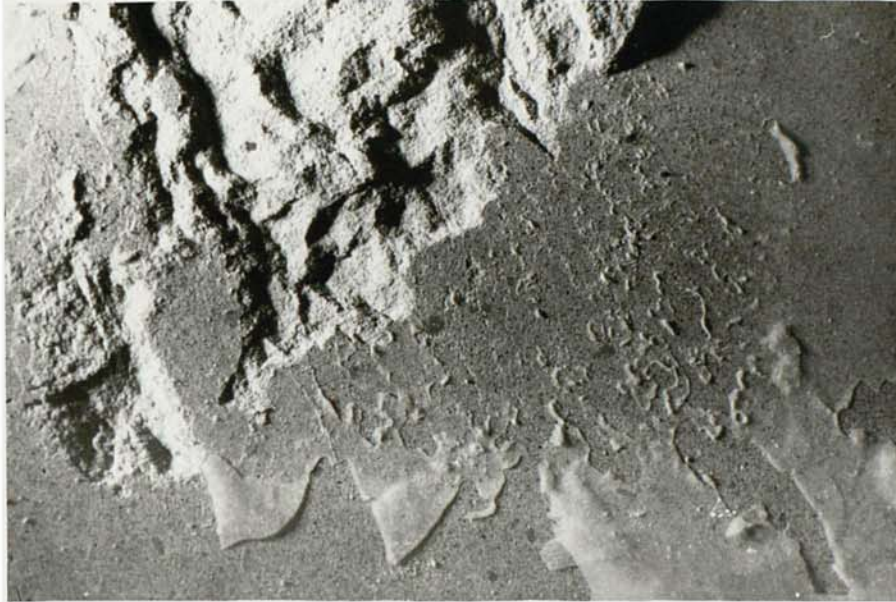
FIGURE 4.14a LOCUS OF FAILURE IN SUPERGLUE
