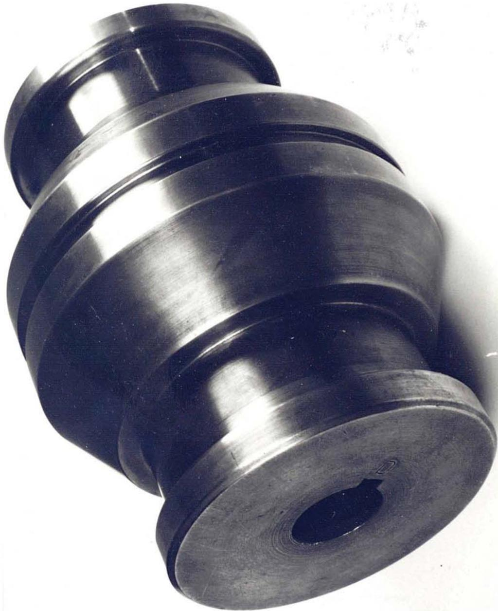
PHOTOGRAPH P5 TOP AND BOTTOM ROLLS OF THE FIRST PASS
