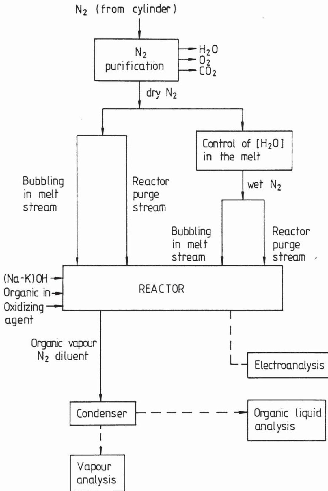
Figure 4-1 Block diagram of equipment for the oxidation of organic vapours in molten salts.
