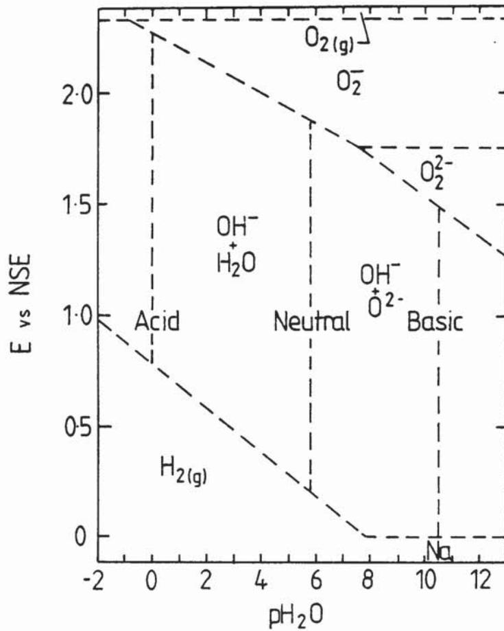
Figure 3-1 Pourbaix diagram for molten (Na, K) OH
