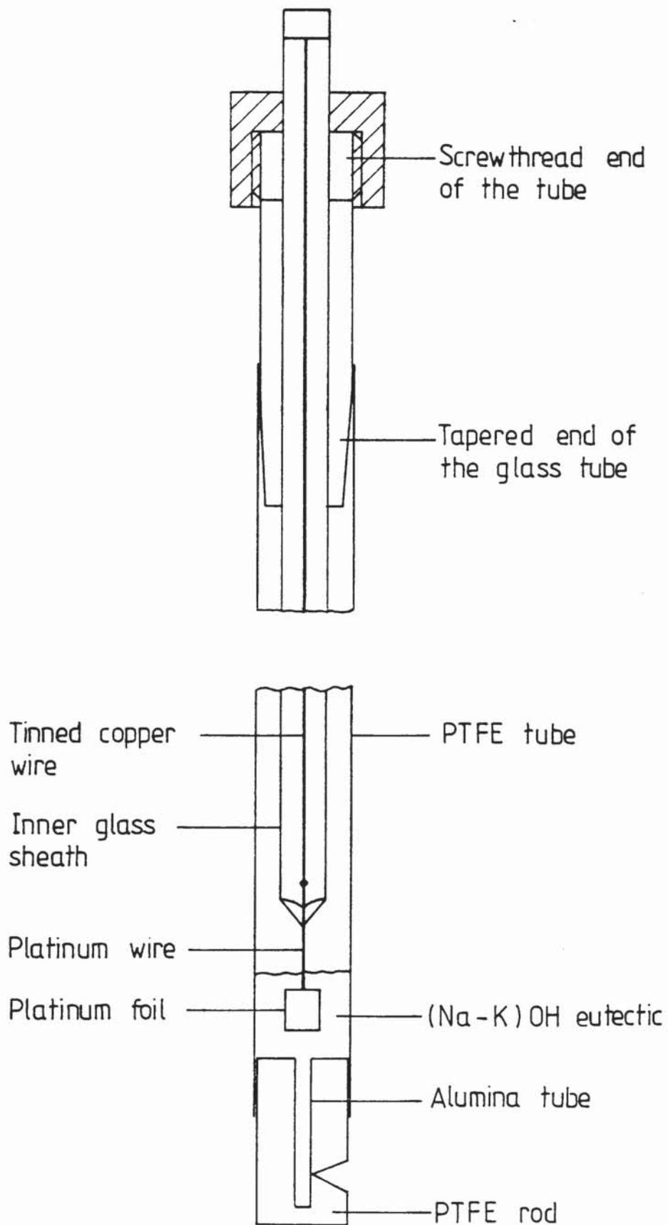
Figure 4-9 Reference and secondary electrodes.
