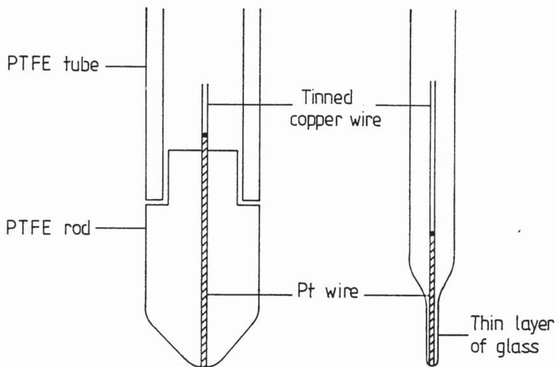
Figure 5-1 The working electrodes used in the preliminary experiments.
