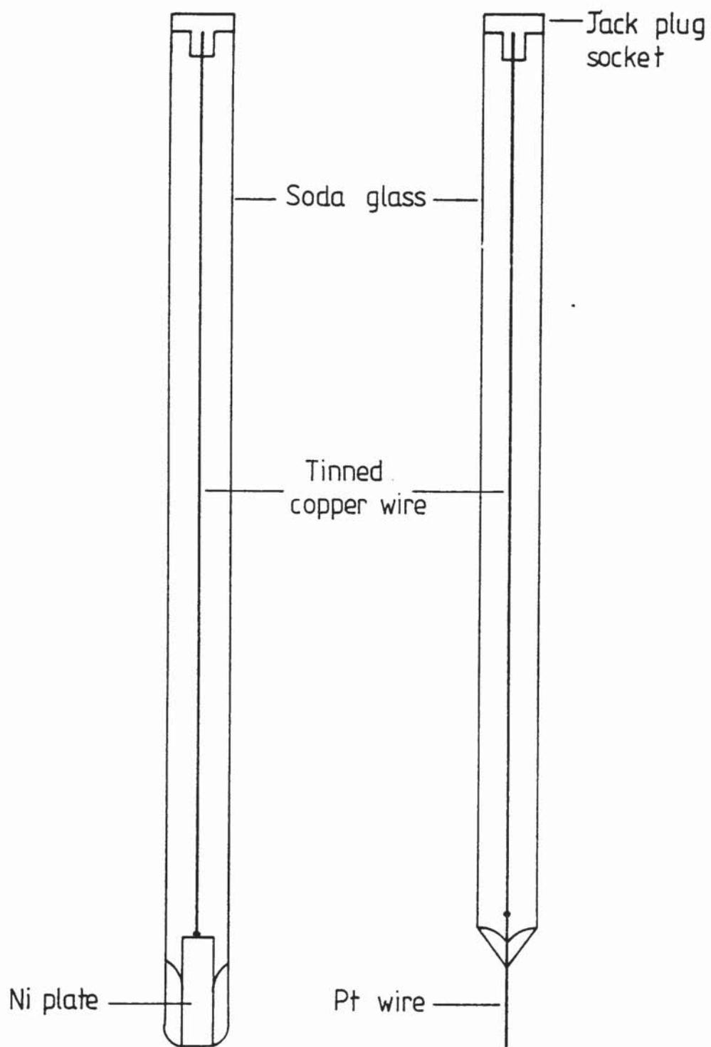
Figure 4-8 Indicator electrodes
