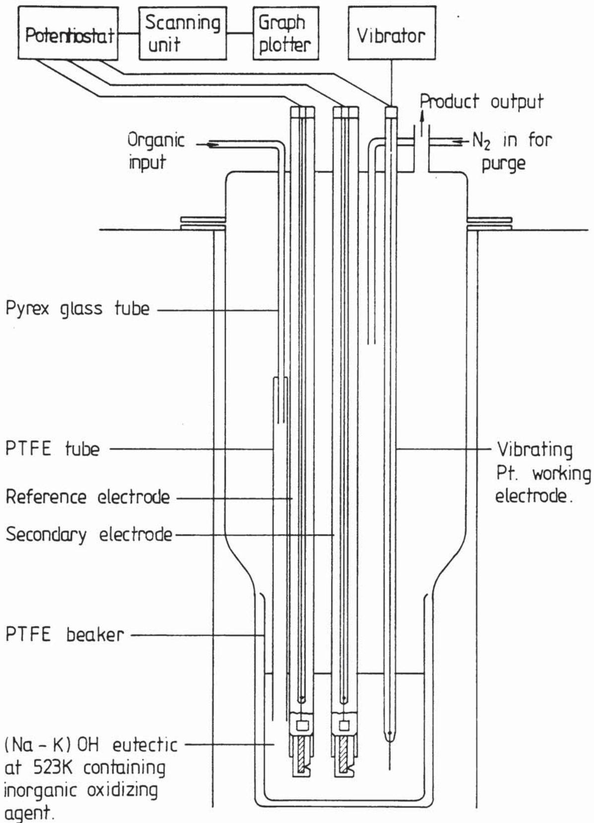
Figure 4-3 Reactor system.
