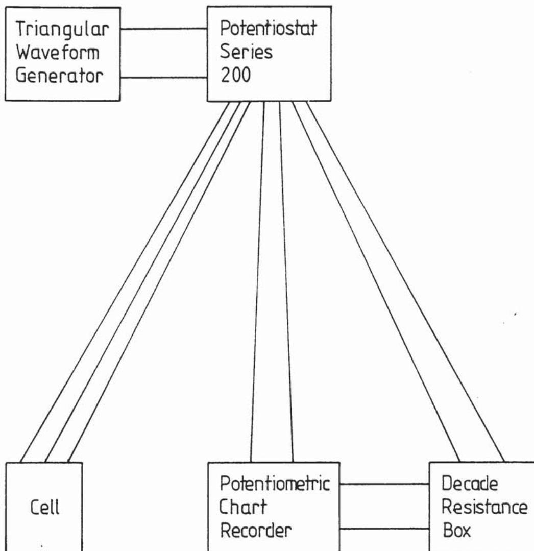
Figure 4-7 Simplified wiring diagram of voltammetric system.
