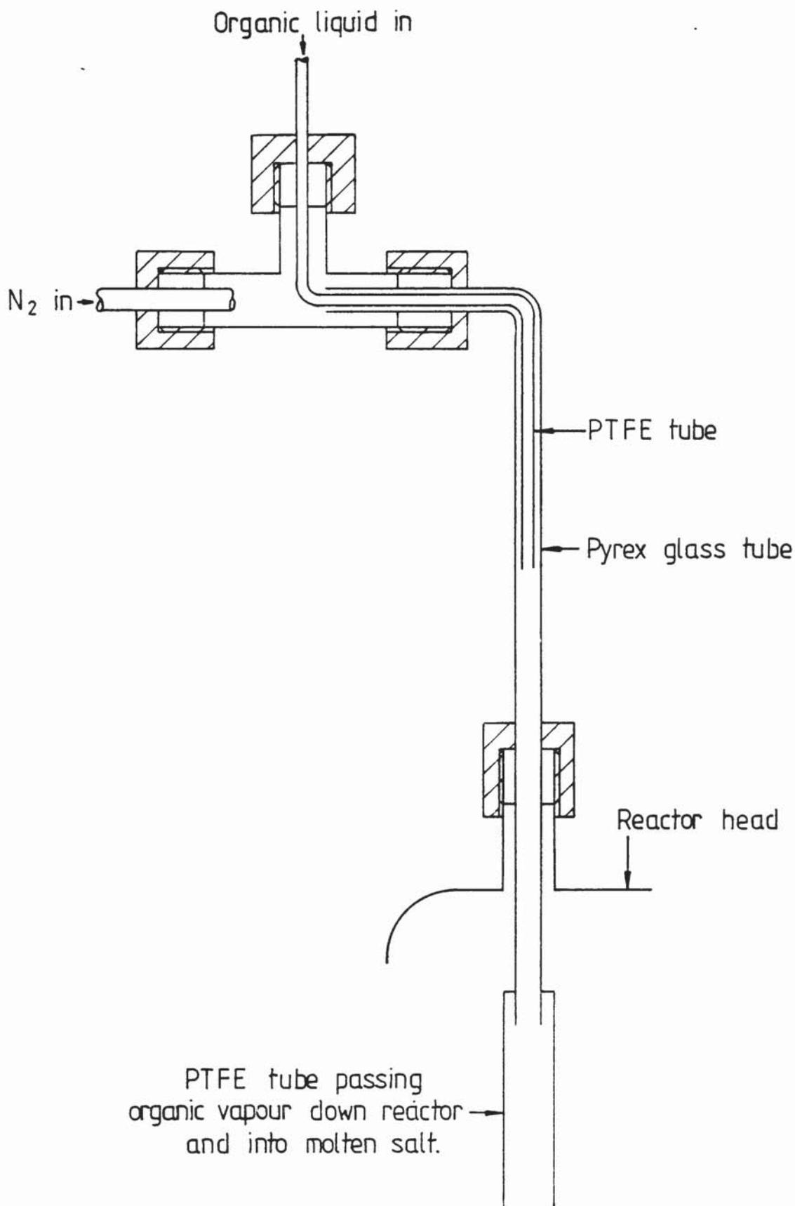
Figure 4-5 Equipment used for injection of organics.
