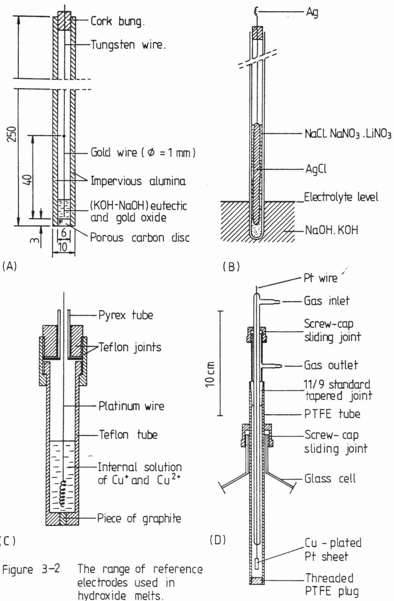
Figure 3-2 The range of reference electrodes used in hydroxide melts.
