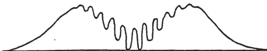
FIGURE 6.9 SIGNAL OBTAINED FROM PARTICLES CROSSING OFF CENTRE OF FRINGE PATTERN
